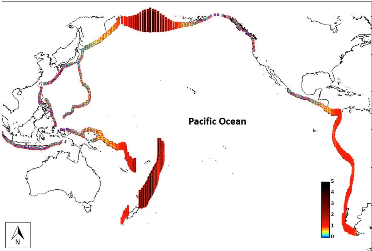
**Figure 9.2** Distribution of tsunami maximum amplitude at a random coastal location in the Pacific Ocean from each of the potential scenarios extracted from NCTR’s propagation data base. A subset of all the scenarios represented can be selected and simulated at high-resolution to arrive at a final PMT for the specific site under investigation
