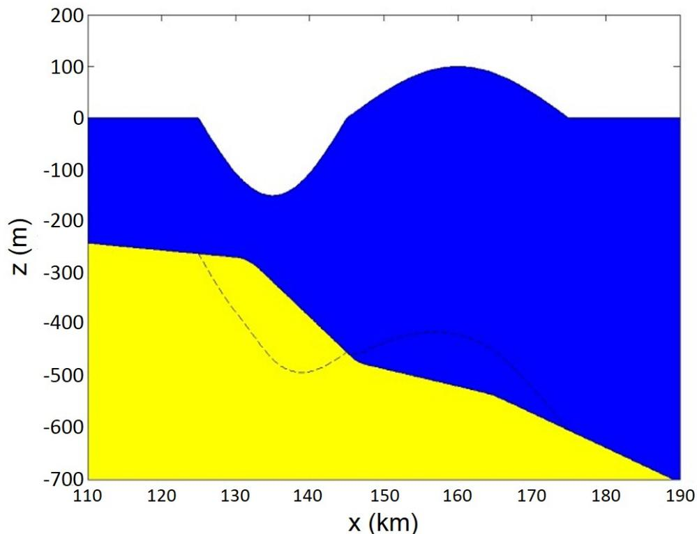
**Figure 7.2** Initial condition for a tsunami generated by a submarine landslide. The "before" landslide profile is given by the solid yellow surface and the "after" landslide profile is given by the black dashed line. The difference in these two profiles results in the initial sea surface elevation profile as shown in solid blue.
