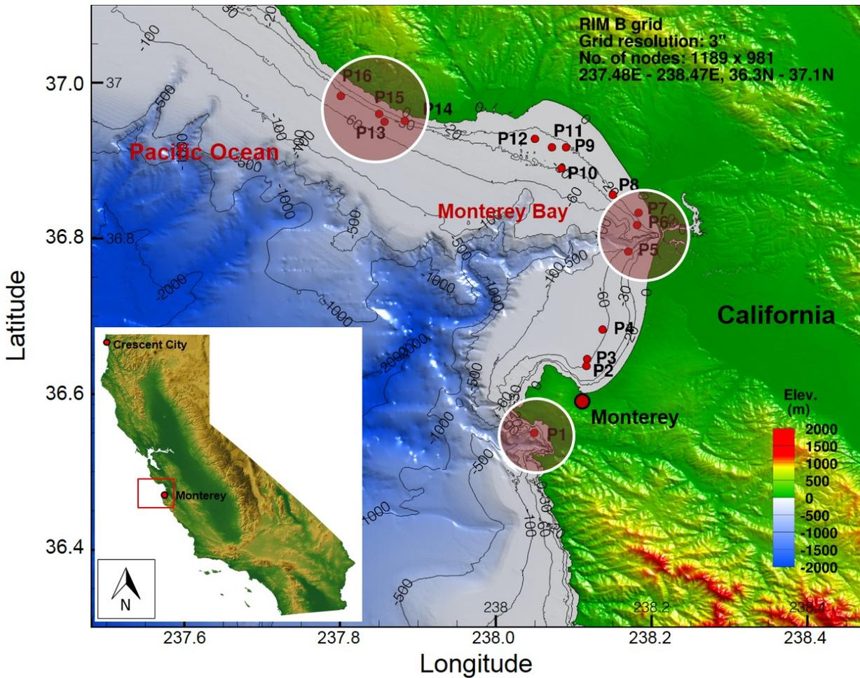
**Figure 10.4** Locations at Monterey Bay, California, where the offshore tsunami heights were obtained (from Thio et al., 2010). The circles are areas of large water depth discrepancies between Thio et al. (2010) and NCTR’s tsunami model.
