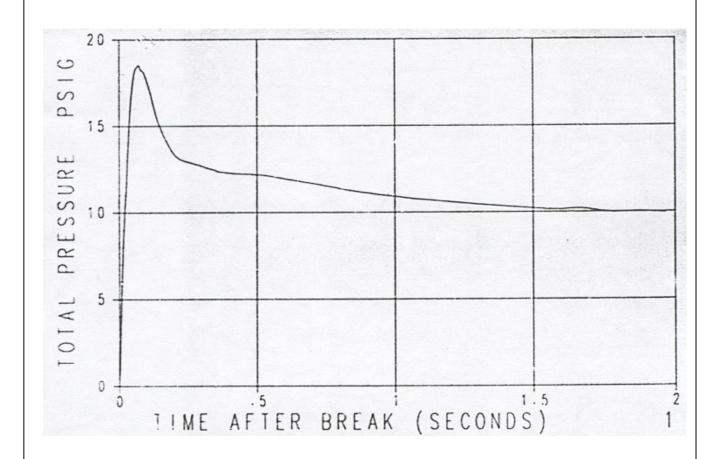
(When using this figure, the differential pressure time history should be increased by an adder of 1.936.)
