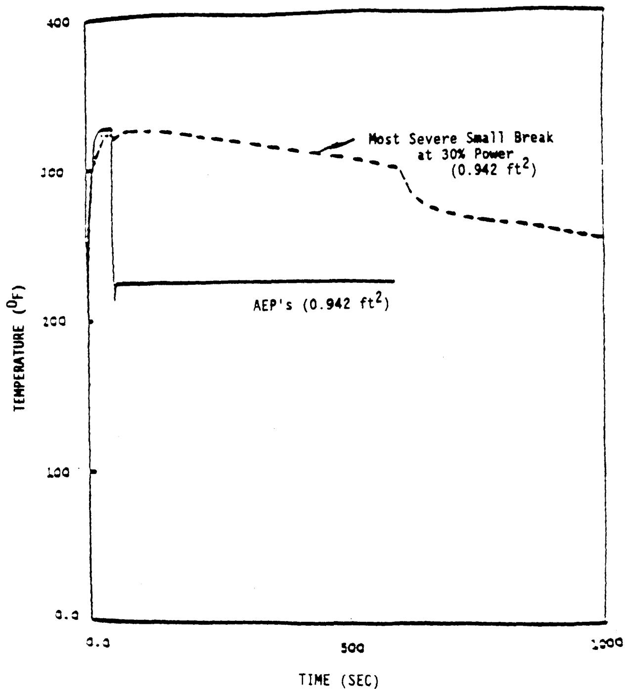
Figure 14.3.4-13 Worst Break-Lower Compartment Temperature Comparison
