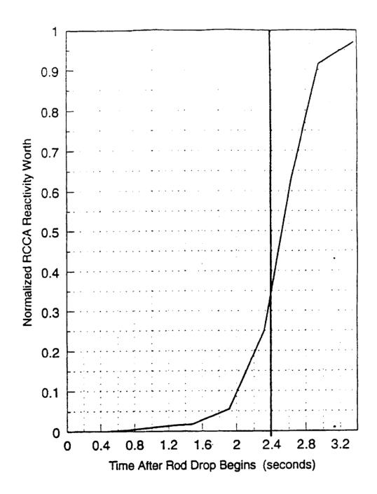
Figure 14.1-5 Trip Reactivity vs. Rod Drop Time
