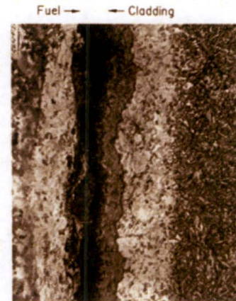
Rare earths → Ferrite → Martensite Optical, Etched, 500×
