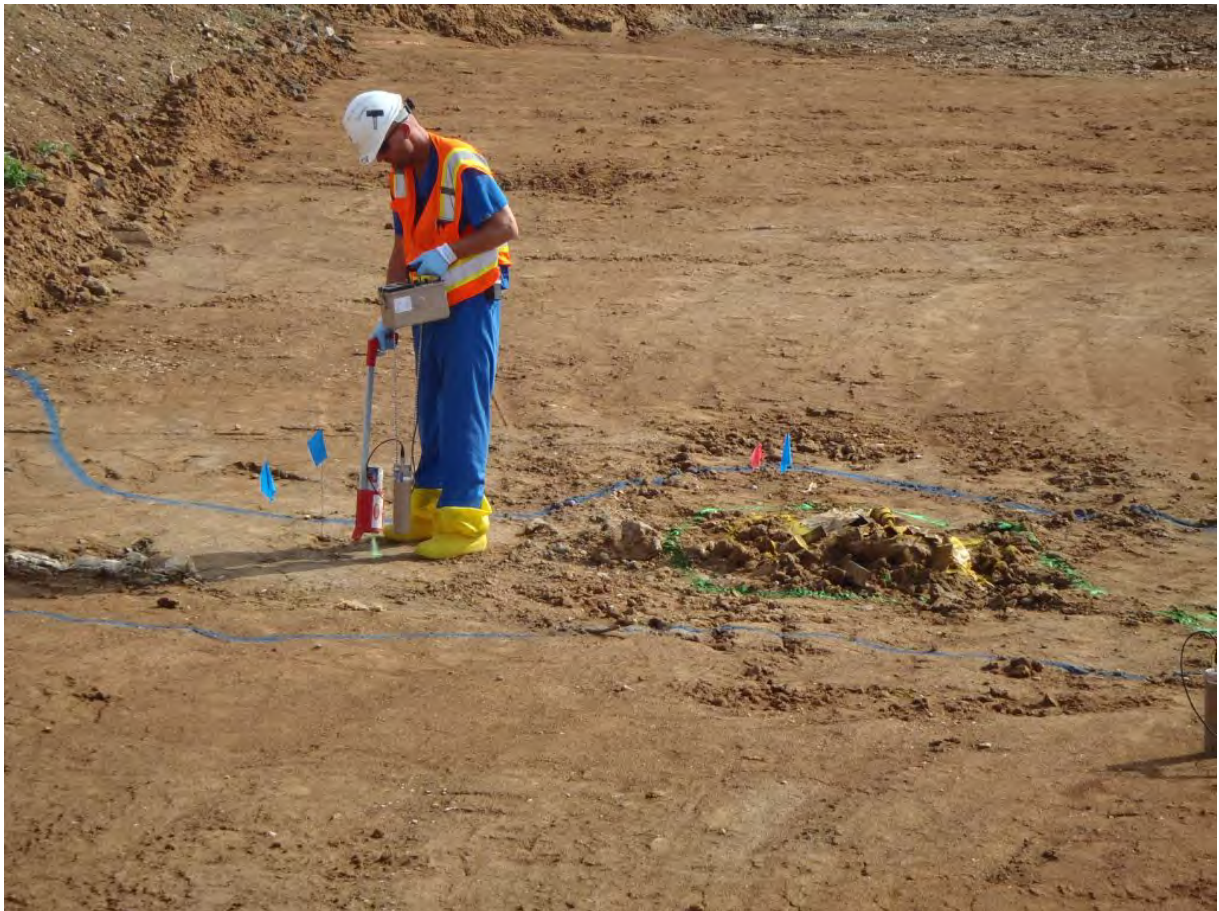
Figure 6 Example of Worker Conducting a Gamma Walkover Survey (GWS) in the Burial Pit Area with a NaI 2 x 2 Detector
