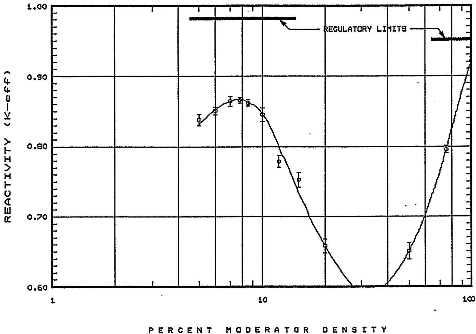
Fig. 1 Variation of new-fuel storage vault reactivity ( $k_{eff}$ ) with water density ( $\rho_{100\%} = 0.998$ ).
