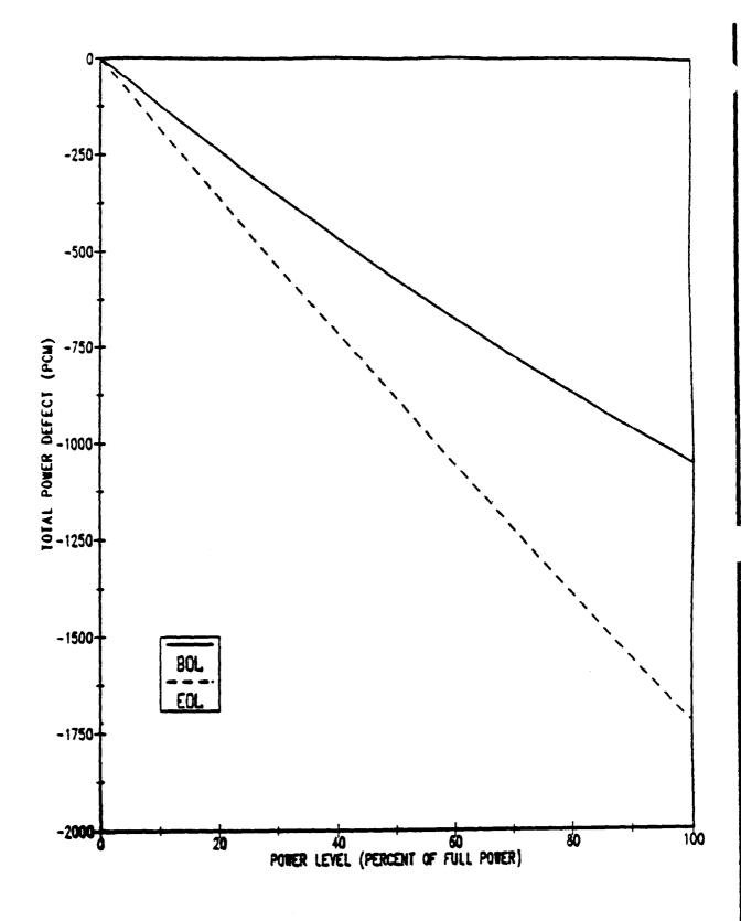
Figure 3.3-34 Example Total Power Defect at BOL and EOL
