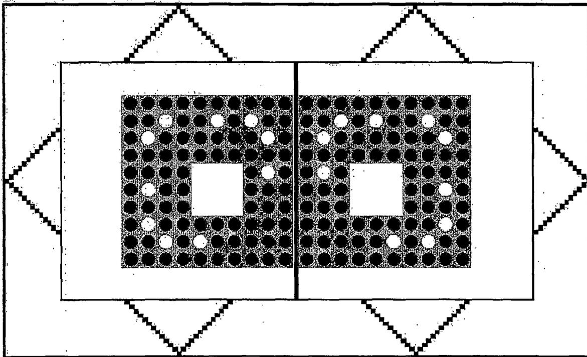
**Figure 4 Assemblies Moved as Close as Physically Possible within Inner Packaging**
