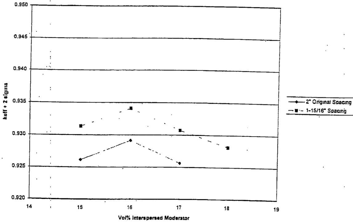
Figure 6.5 Container Spacing and Interspersed Moderator Sensitivity Study for Fuel Category 6 Inside SP-1/SP-2 Inner Containers, 8x13x1 Array (104 containers), Damaged Conditions
