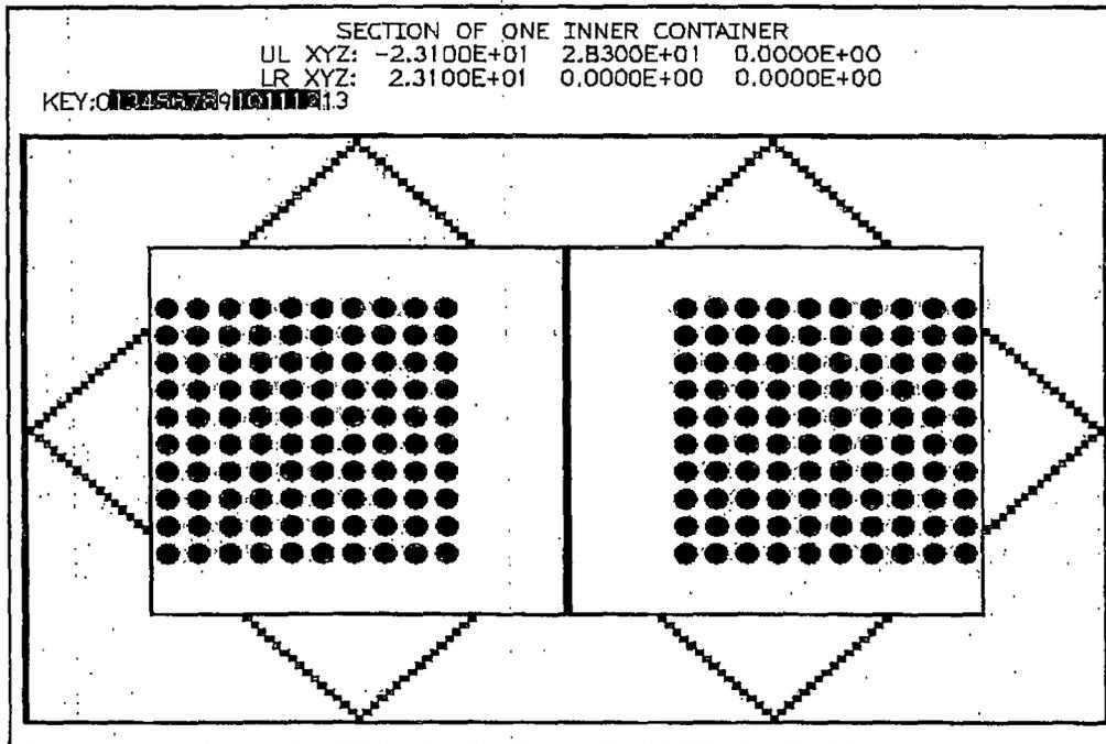
CASMO-3G was also used to calculate  $k$ -inf for several cases. The steel and moderation were "smeared" together in the various regions of the CASMO model. The CASMO model also had the assemblies shifted to the outer edges of their baskets. The arrays modeled were either infinite or  $8 \times 13 \times 1$ .
