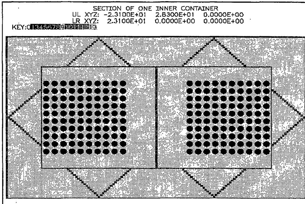
CASMO-3G was also used to calculate  $k$ -inf for various fuel types. The steel and moderation were "smeared" together in the various regions of the CASMO model. The CASMO model also had the assemblies shifted to the outer edges of their baskets. The arrays modeled were either infinite or  $8 \times 13 \times 1$ .
