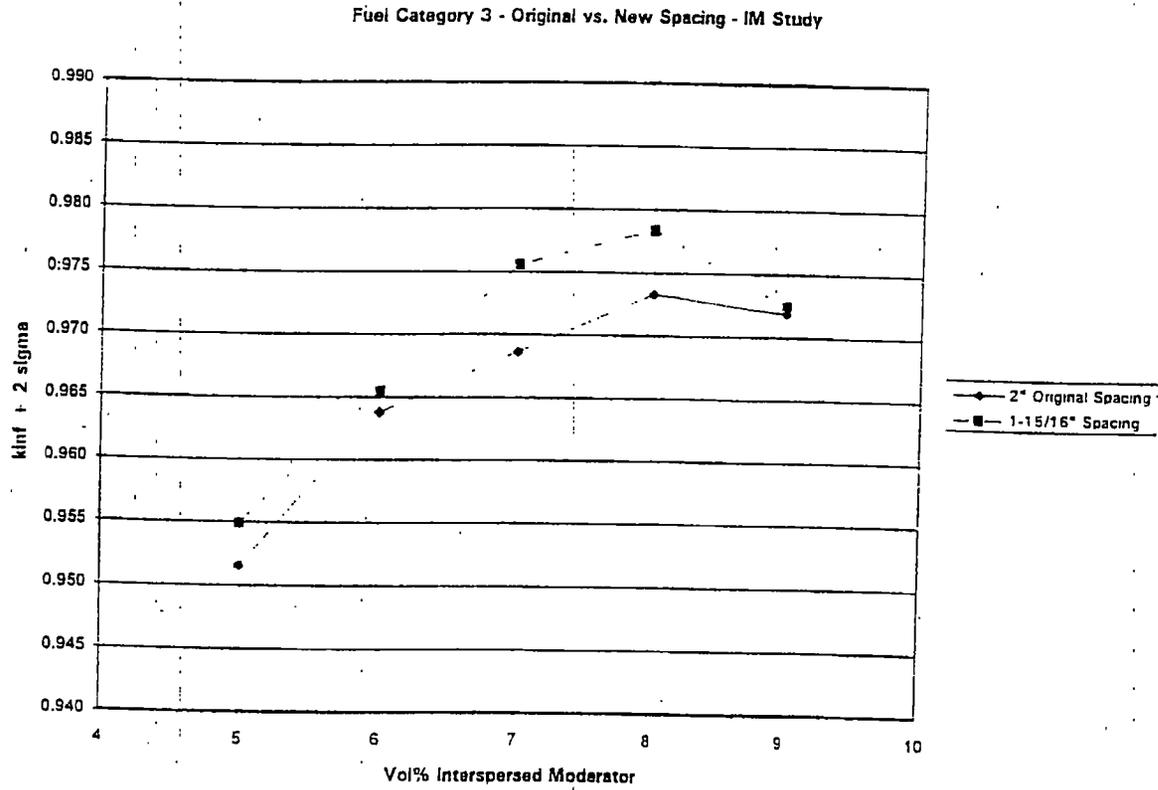
Figure 6.3 Container Spacing and Interspersed Moderator Sensitivity Study for Fuel Category 3 Inside SP-1/SP-2 Inner Containers, Infinite Array, Damaged Conditions
