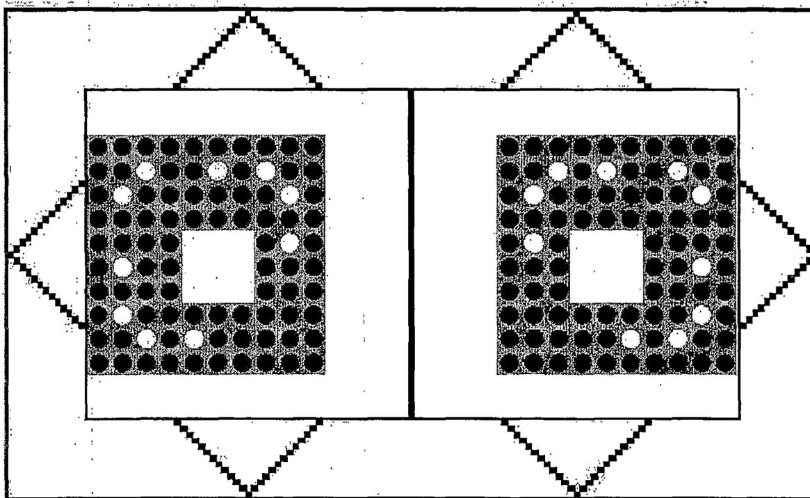
**Figure 5 Assemblies Moved as Far Apart as Physically Possible within Inner Packaging**
