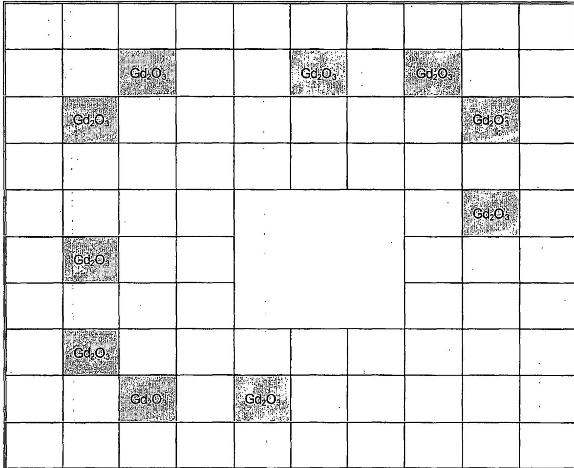
Figure 1 Gd<sub>2</sub>O<sub>3</sub> Rod Placement which Produces Most Reactive Assembly (Reference 8)
