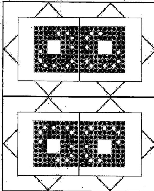
**Figure 12 Assemblies as Close as Physically Possible within Inner Packaging and Asymmetric Gd<sub>2</sub>O<sub>3</sub> Rods in the Assemblies in Each Group of Two Vertically Adjacent Inner Packages Facing Towards the Inside of the Group**
