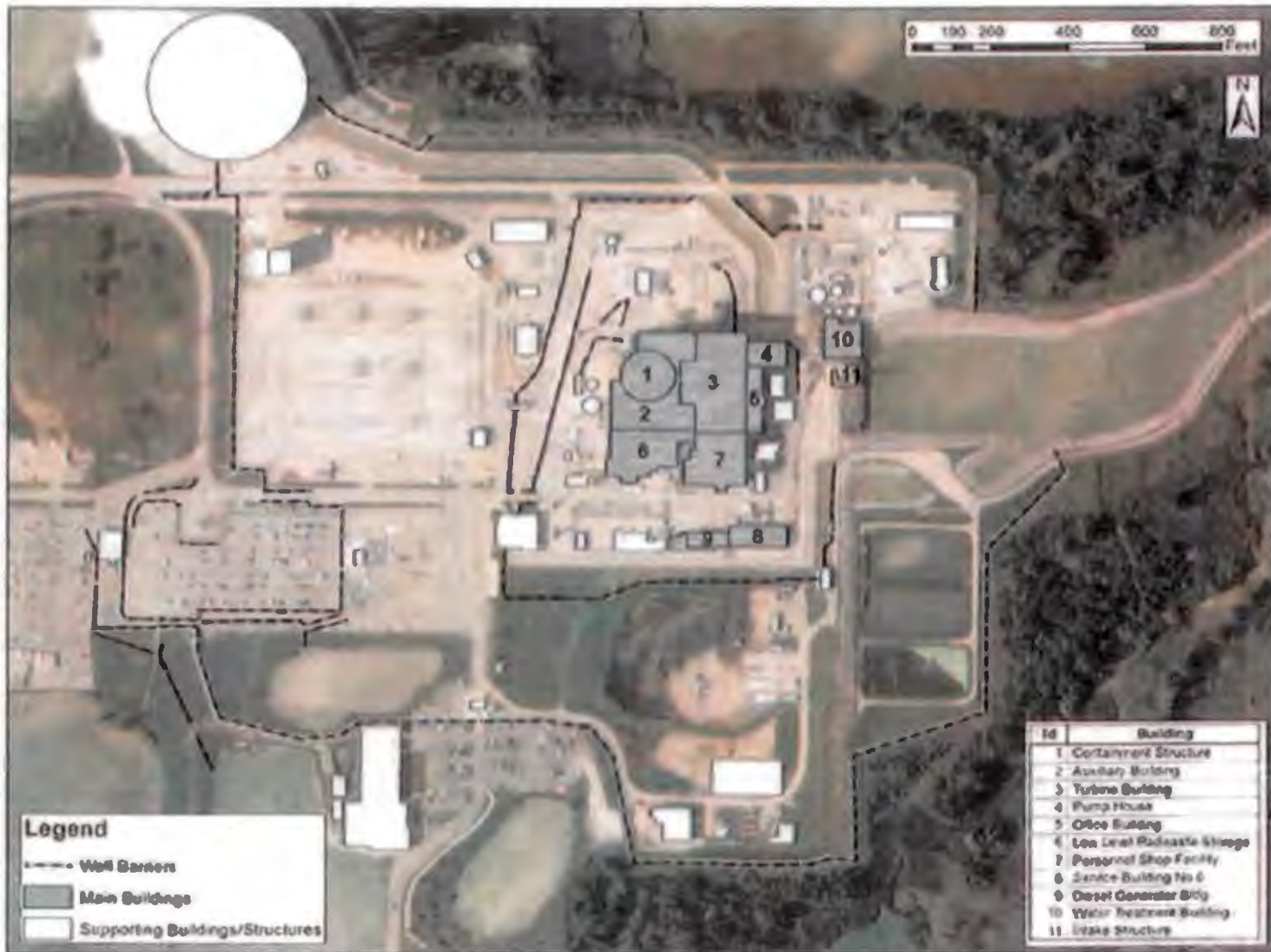
Figure 3.1-1. Key features of the Davis-Besse site that were depicted in the FLO-2D PRO computer model used to evaluate LIP. From FENOC (2015a).
