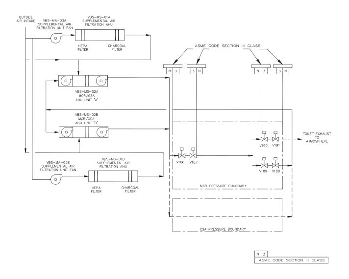
Figure 2.7.1-1 (Sheet 1 of 2) Nuclear Island Nonradioactive Ventilation System
