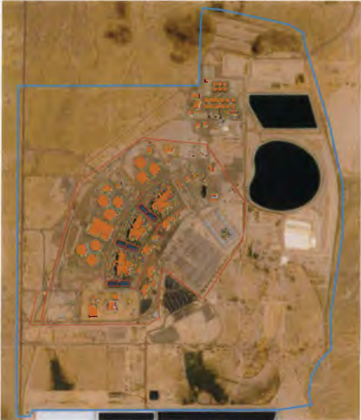
Figure 3.2-3. FLO-2D Model Domain (in blue) for the LIP Flooding Evaluation. VBS shown in red, buildings in orange.
