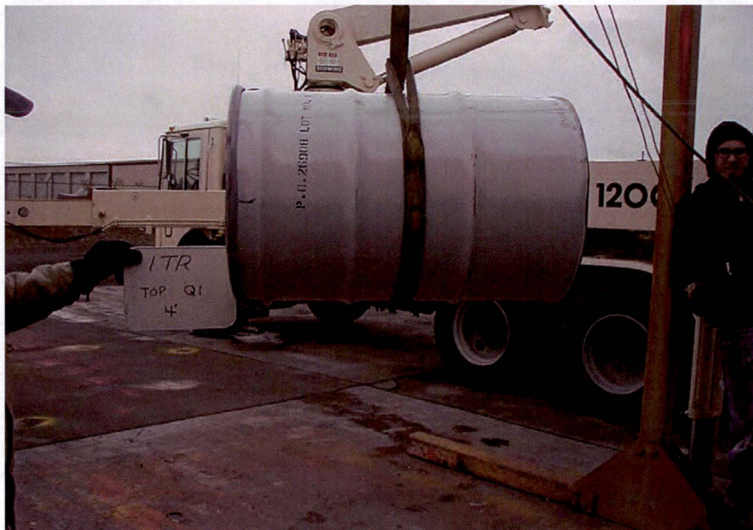
Figure 2.12.1-4 - S300 Side Four-Foot Free Drop
