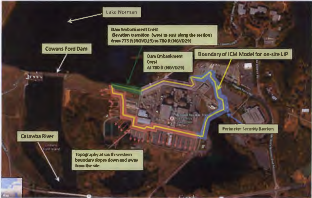
Figure 3.2-1. ICM Model Area and Boundaries for the On-Site LIP Analysis (Derived from Duke, 2014d and Duke, 2014e)
