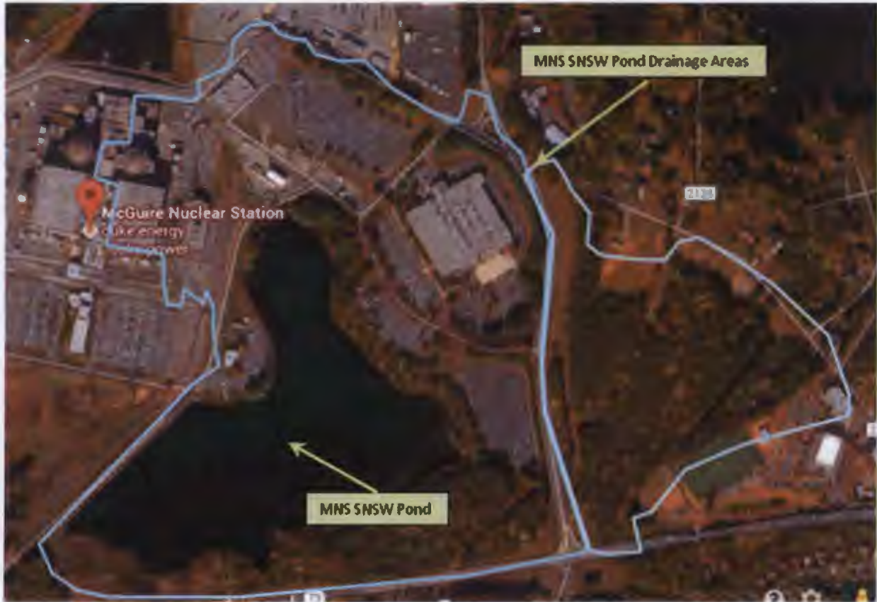
Figure 3.2-2. Drainage Area of the Standby Nuclear Service Water Pond for the On-Site LIP Analysis (Derived from Duke, 2014h)
