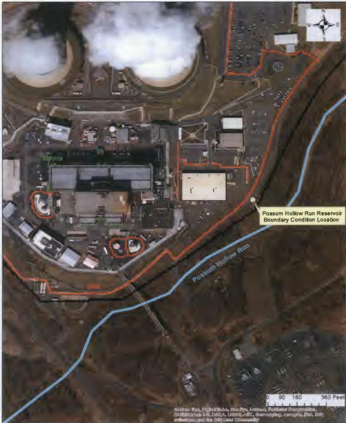
Figure 3.2-2. FLO-2D Model Boundary in the Powerblock Area
