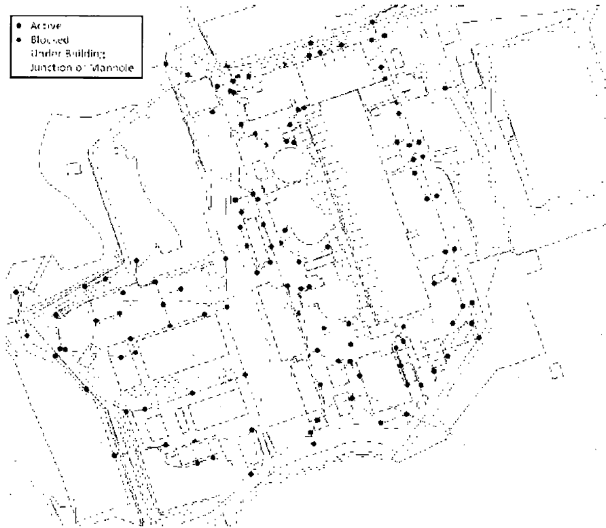
Figure 3.2-6. ONS Yard Catch Basins (adapted from the Revised FHRR (Duke, 2015b, Figure A-10-A))
