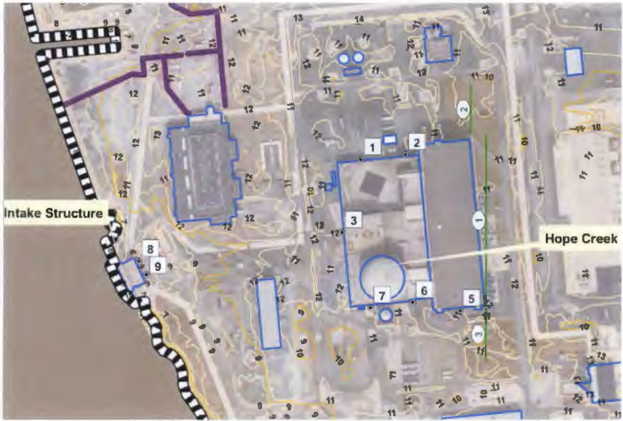
Figure 3.2-4. Critical Door Locations Used for Local Intense Precipitation Analysis at the HCGS Site (modified detail from FHRR Figure 2.1-3 (PSEG, 2014a))
