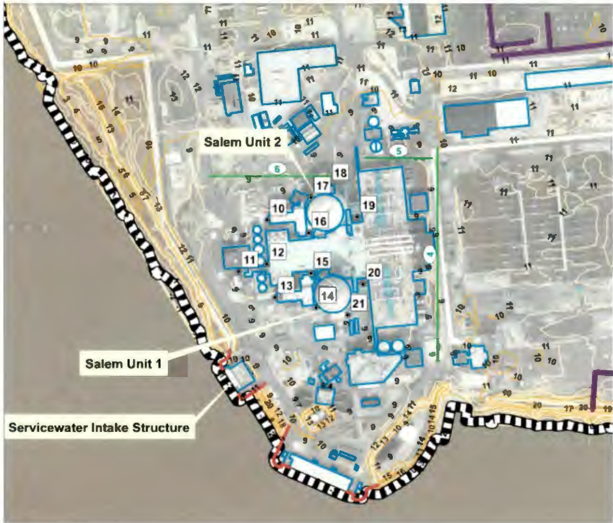
Figure 3.2-4. Critical Door Locations Used for Local Intense Precipitation Analysis at the Salem Site (modified detail from PSEG, 2014a, FHR Figure 2.1-3)
