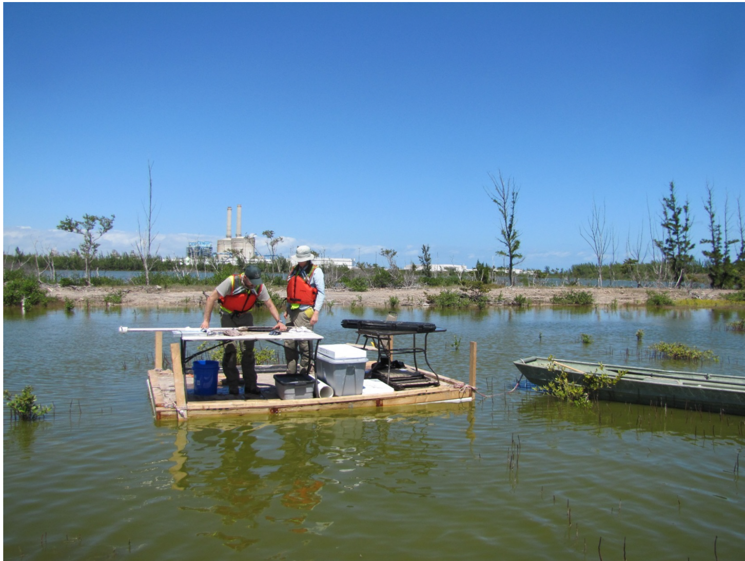
Figure 2-5 Anchored Coring Platform Prepared for Florida Power & Light Miami-Dade County, Florida
