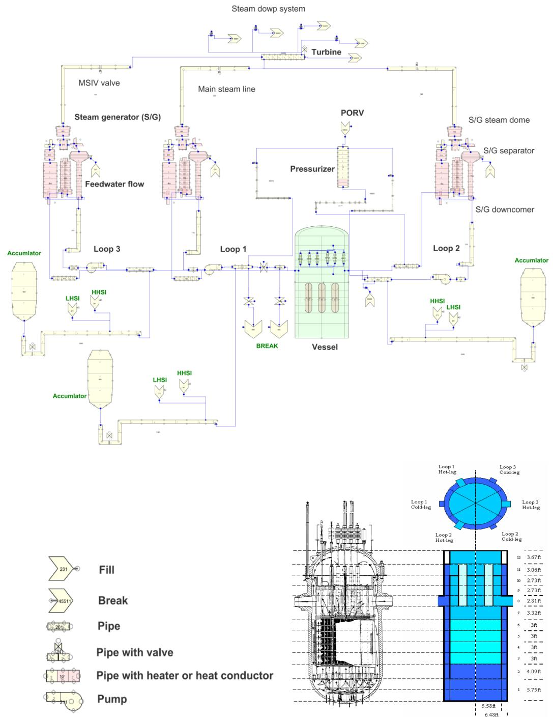
**Figure 2 The LBLOCA TRACE Model of Maanshan NPP**
