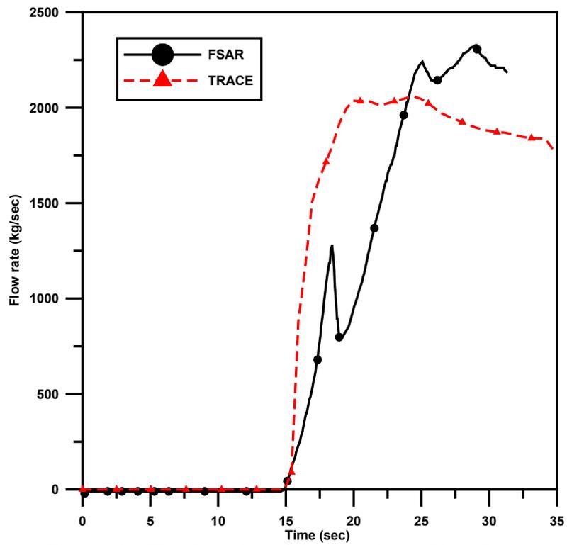
Figure 6 The Results of Accumulator Flow Rate
