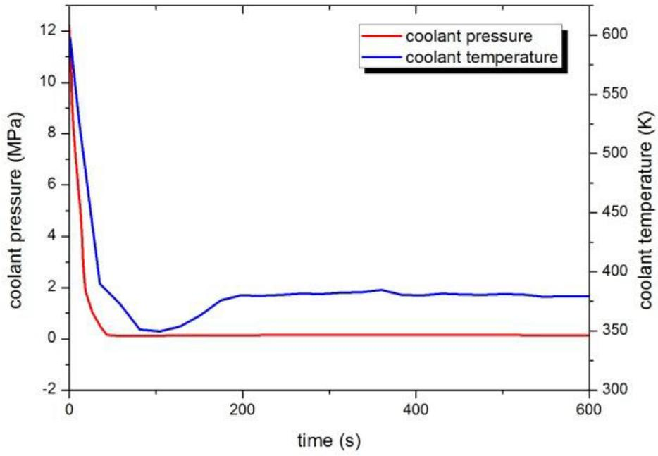
Figure 12 The Coolant Pressure and Temperature History at T01 Zone from TRACE
