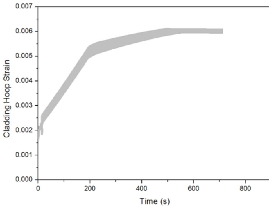
**Figure 20 The 59 Cladding Hoop Strains as A Function of Time**
