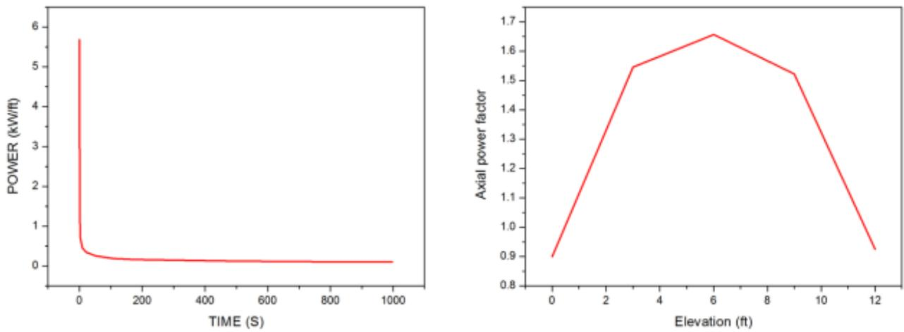
Figure 11 The Power History after Scram from TRACE (Left) and the Axial Power Shape of the Fuel Rod (Right)
