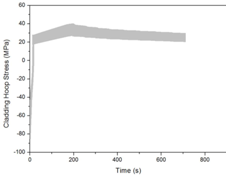
**Figure 21 The 59 Cladding Hoop Stresses as A Function of Time**
