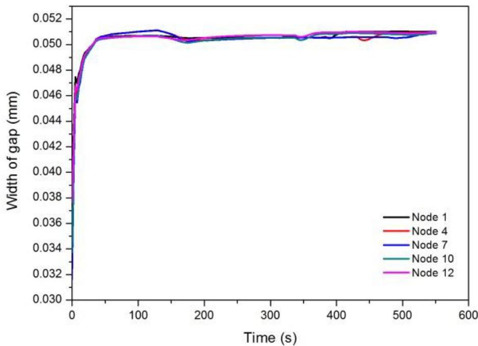
**Figure 13** The Variations of Gap Width in the Rod during Transient at T03 Zone
