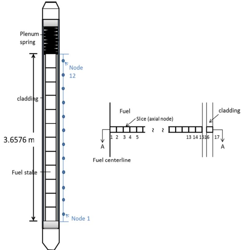
**Figure 9 The Schematic of Fuel Rod Geometry In FRAPTRAN**
