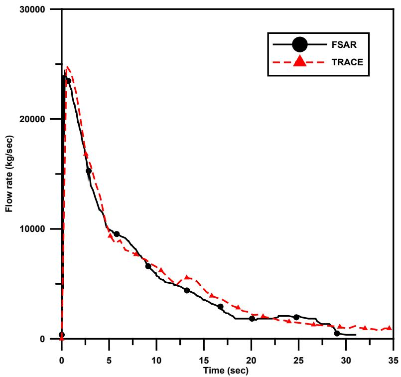
**Figure 5 The Results of Break Mass Flow Rate**
