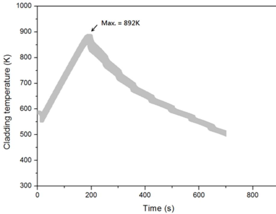
**Figure 19 The 59 Cladding Temperatures as A Function of Time**
