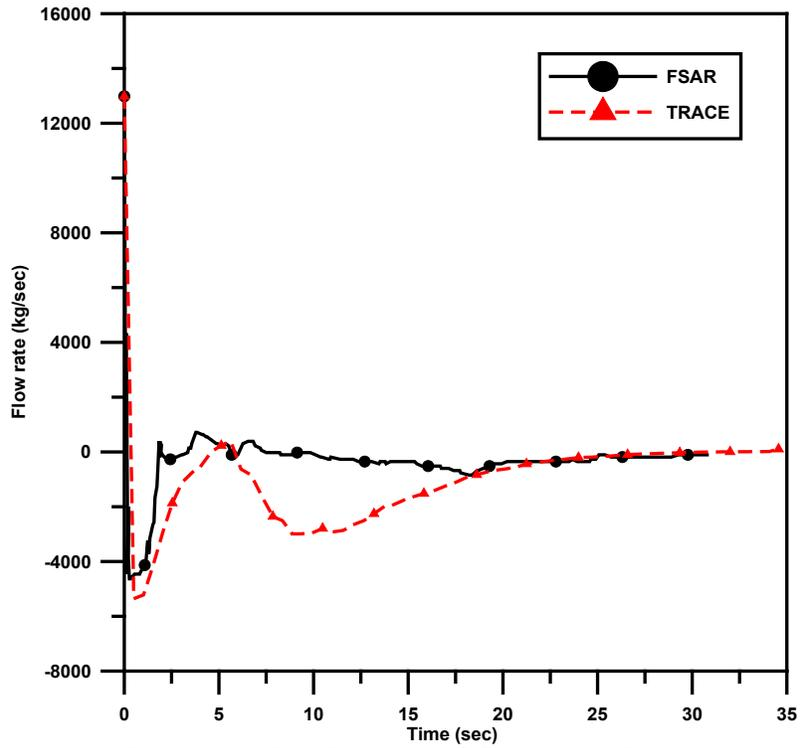
Figure 7 The Results of Core Inlet Flow
