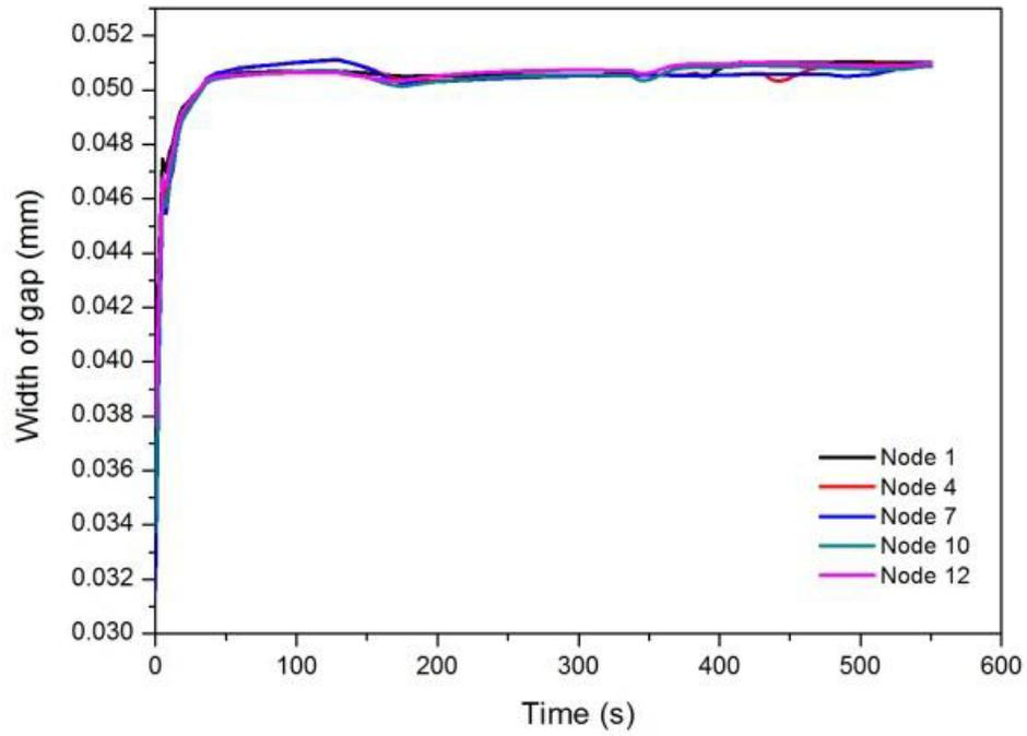
**Figure 13 The Variations of Gap Width in the Rod during Transient at T03 Zone**
