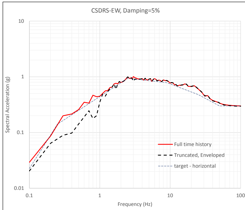
Figure 22 Comparison of Response Spectrum between Full Duration and Truncated Duration for CSDRS-EW Compatible Time History
