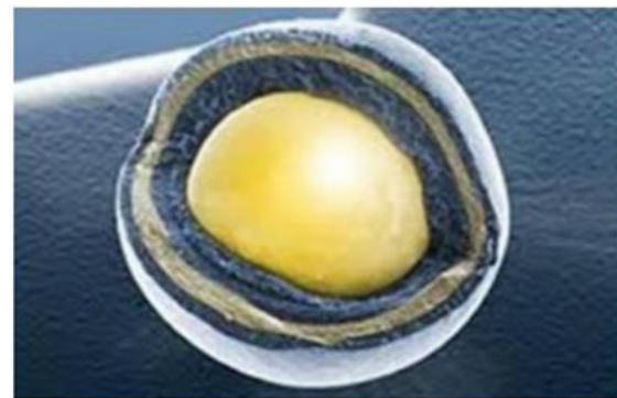
TRISO coated particle fuel
