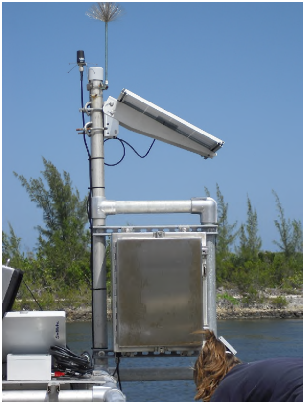
Close-up photo of automated station panel.
