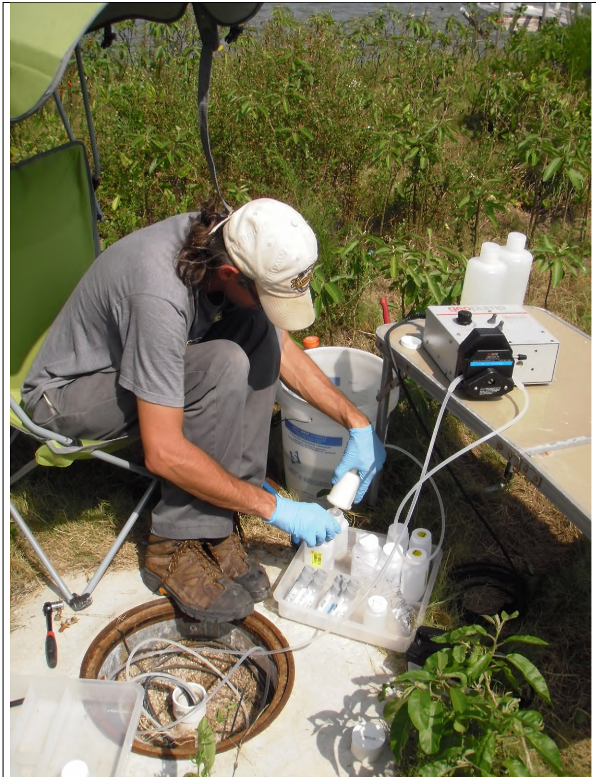
Figure 3.1-1. Typical Groundwater Field Sampling Setup.
