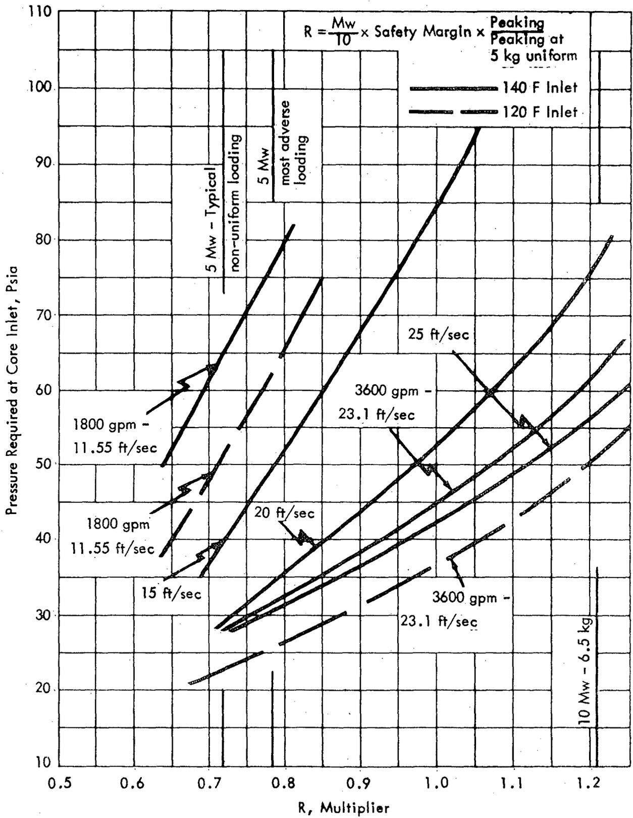
Figure 5.6 Effect of Multiplier R on Coolant Conditions Required to Suppress Boiling
