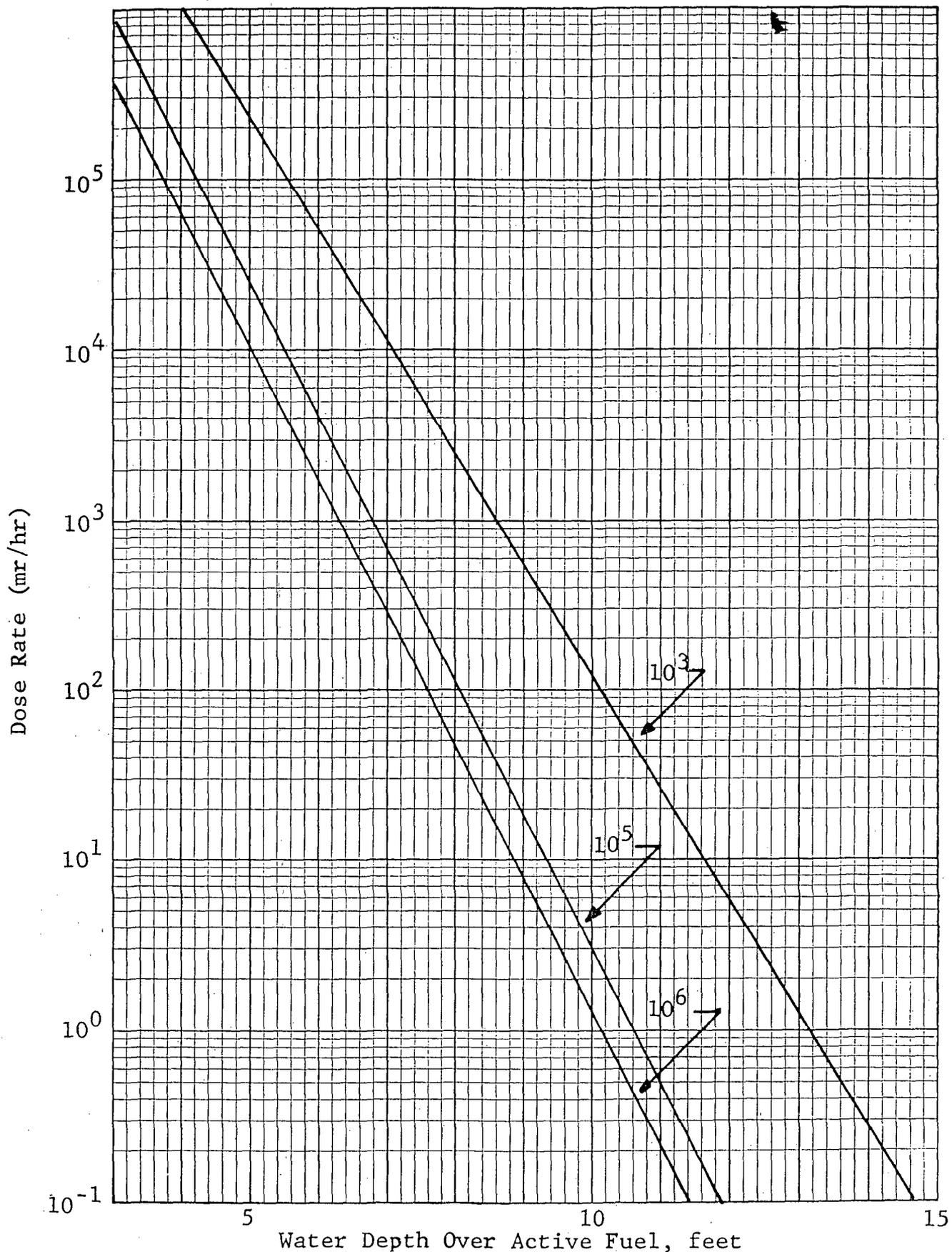
Figure 6.8 Spent Fuel Element Dose Rate Through Water Shielding as a Function of Fission Product Decay Time-Vertical Element (400 MWD Operation)
