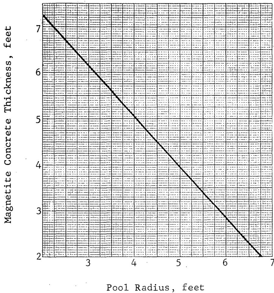
Figure 6.3 Magnetite Concrete Biological Shielding Requirements versus Effective Pool Radius to Achieve One-Tenth of Dose Rate Criteria from Fast Neutron Dose (Reactor Power 10 MW)
