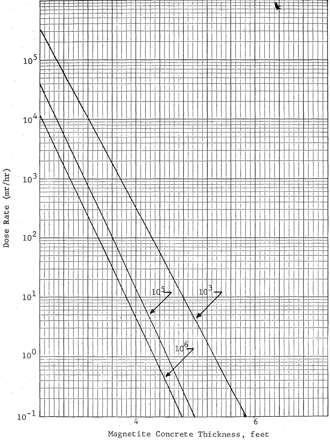
Figure 6.5 Spent Fuel Element Dose Rates Through Magnetite Concrete Shielding for Four Elements as a Function of Fission Product Decay Time (400 MWD Operation)
