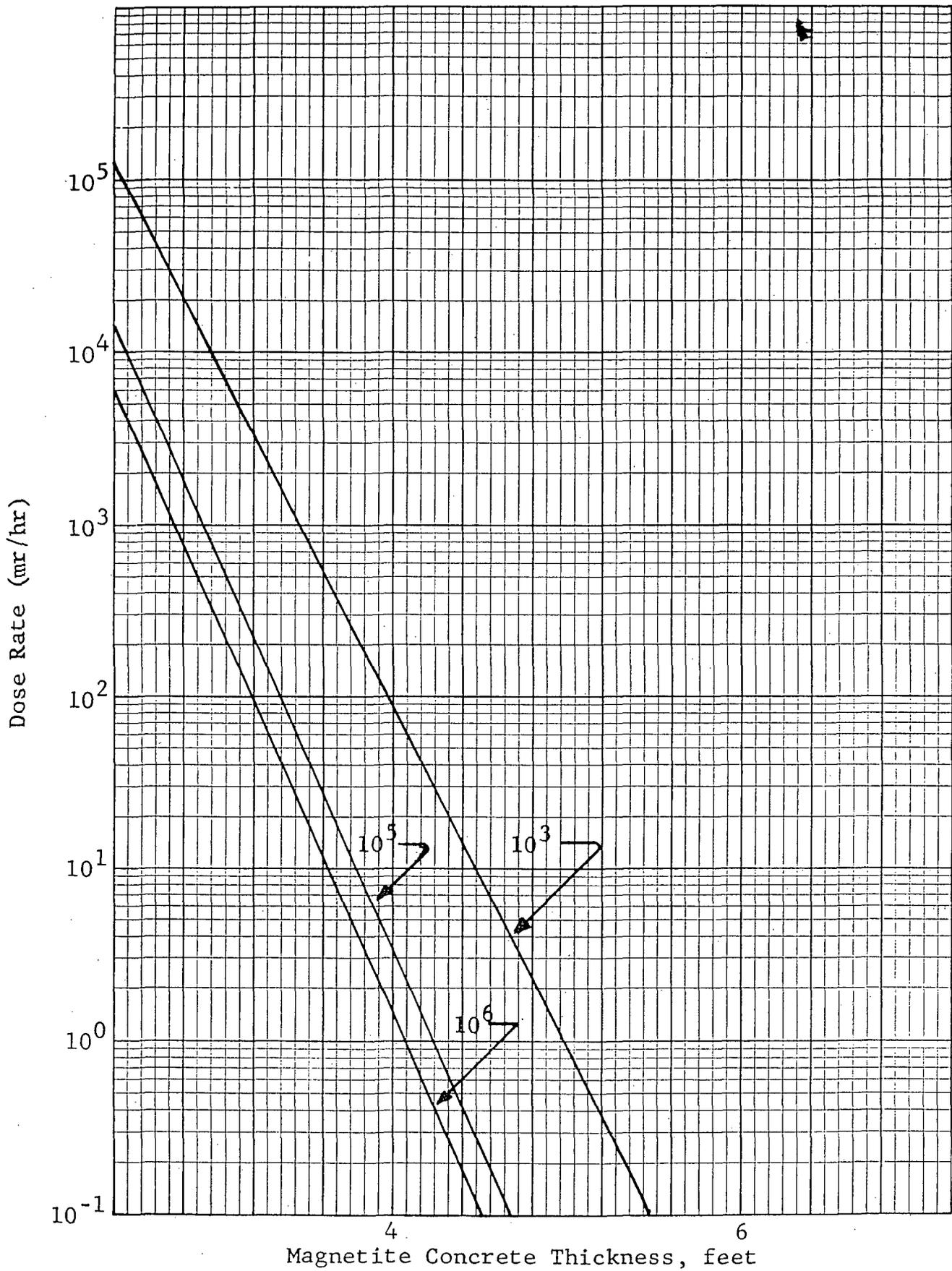
Figure 6.4 Spent Fuel Element Dose Rates Through Magnetite Shielding for a Single Element as a Function of Fission Product Decay Time (400 MWD Operation)
