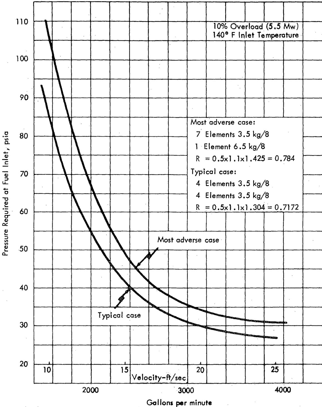
Figure 5.4 Effect of Non-Uniformity of Fuel Loading at 5 Megawatts
