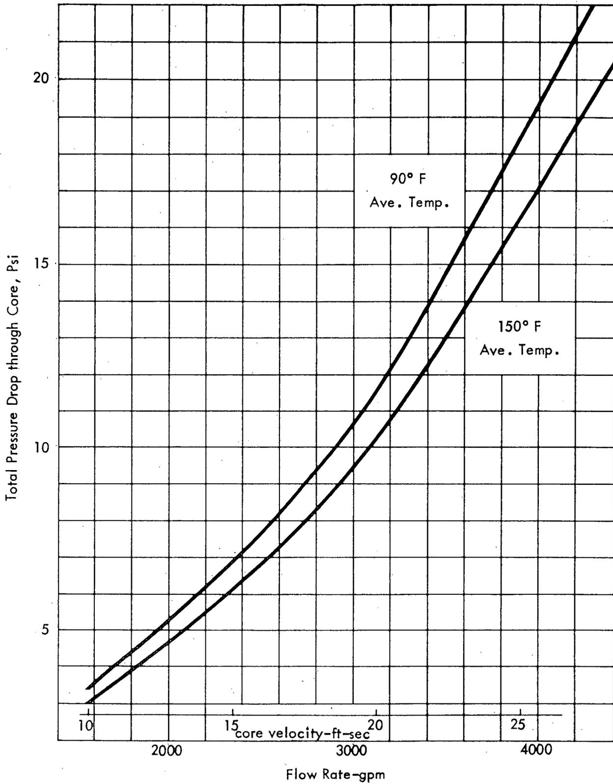
Figure 5.7 Total Pressure Drop Across Fuel Elements
