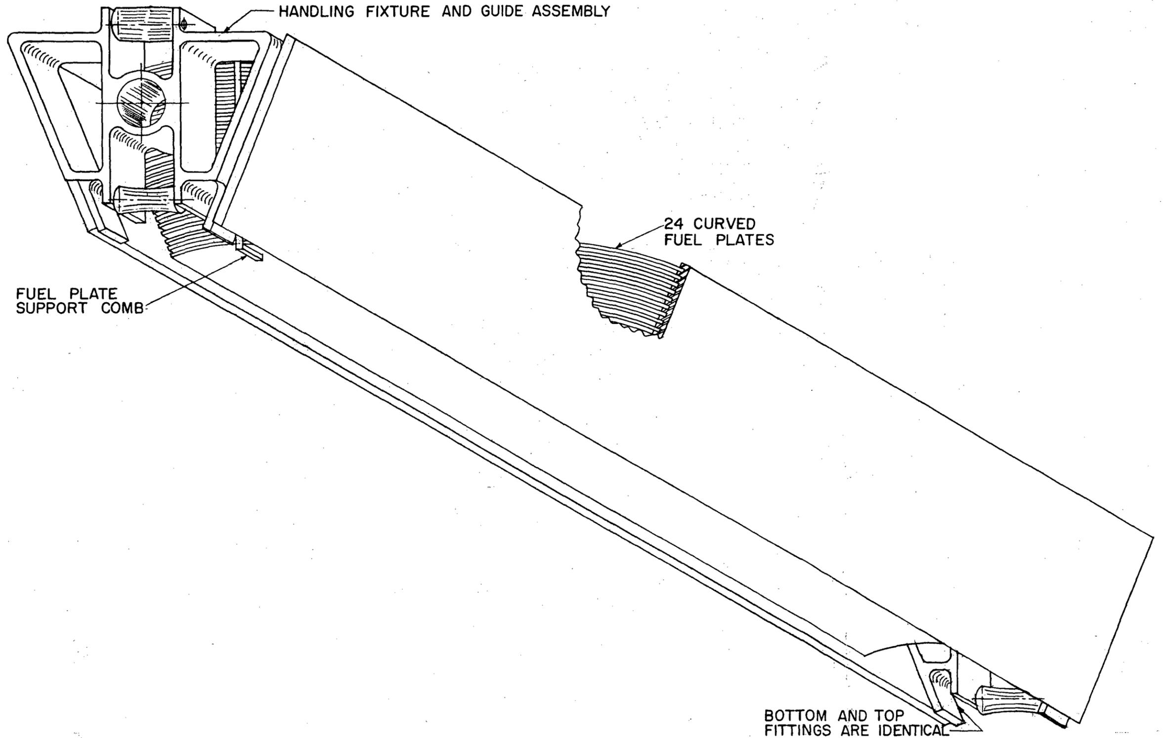
FIGURE 4.3 FUEL ASSEMBLY—PICTORIAL VIEW
