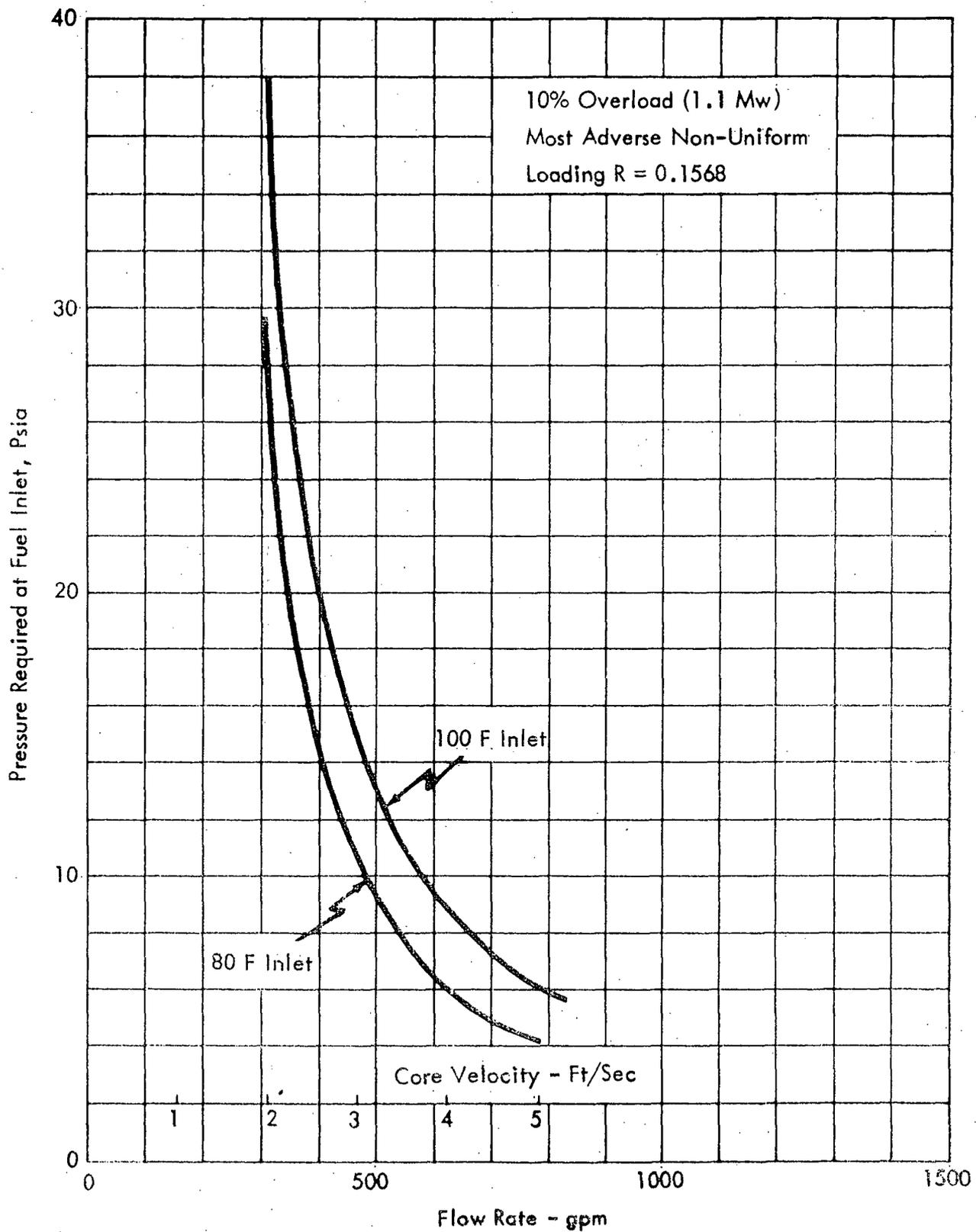
Figure 5.5 Coolant Conditions Required to Suppress Boiling at 1 Megawatt
