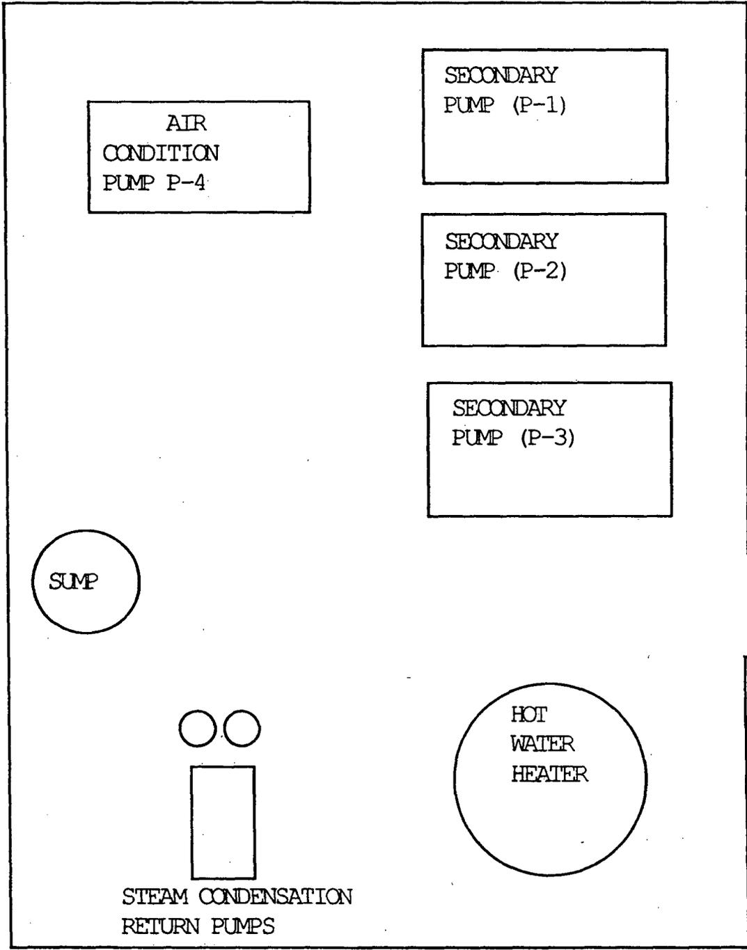
Figure 3.9 Cooling Tower Below Grade Plan
