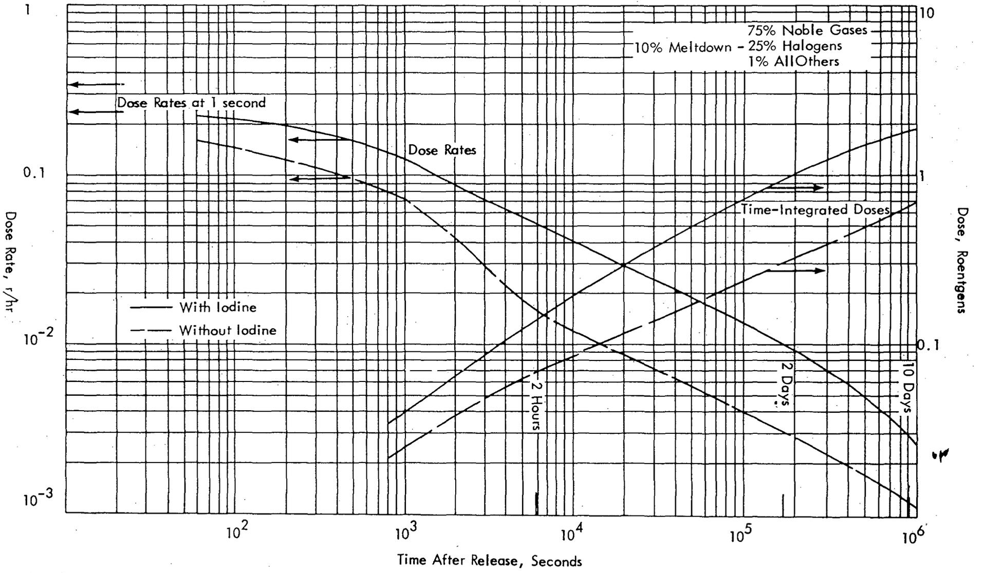
Figure 13.2 External Gamma Exposure From Cloud at 1000 Feet
