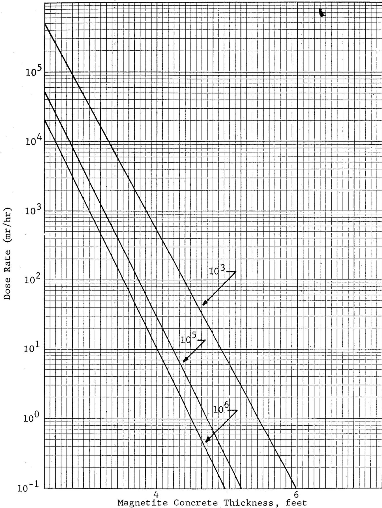
Figure 6.6 Spent Fuel Element Dose Rates Through Magnetite Concrete Shielding for Eight Elements as a Function of Fission Product Decay Time (400 MWD Operation)
