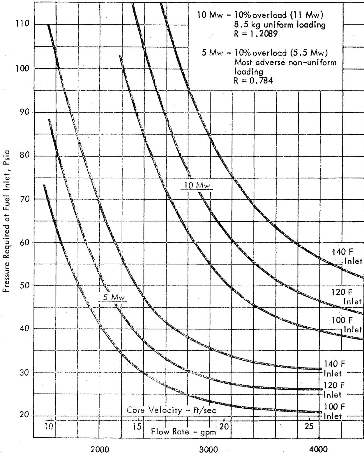
Figure 5.3 Coolant Conditions Required to Suppress Boiling
