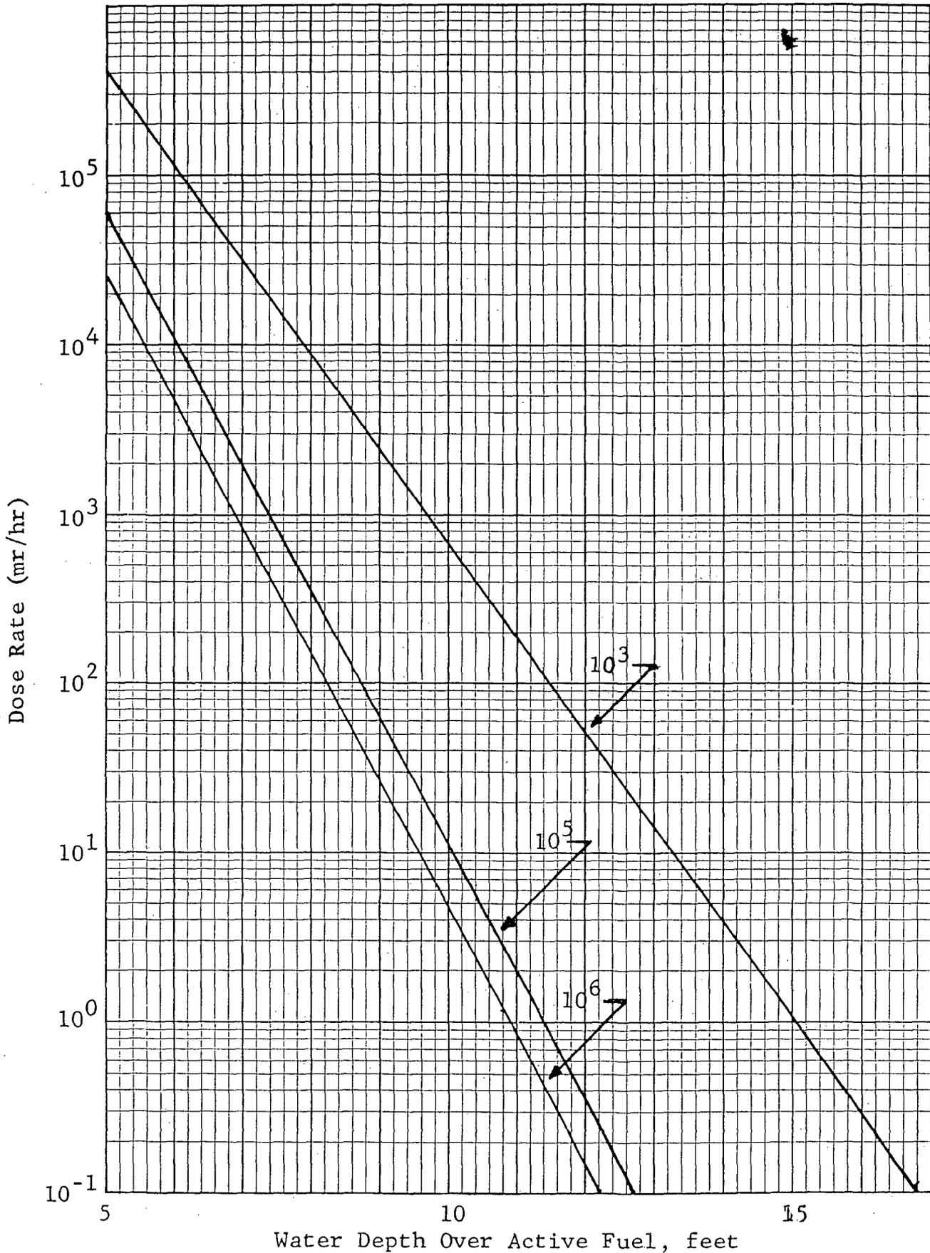
Figure 6.7 Spent Fuel Element Dose Rate Through Water Shielding as a Function of Fission Product Decay Time-Horizontal Element (400 MWD Operation)
