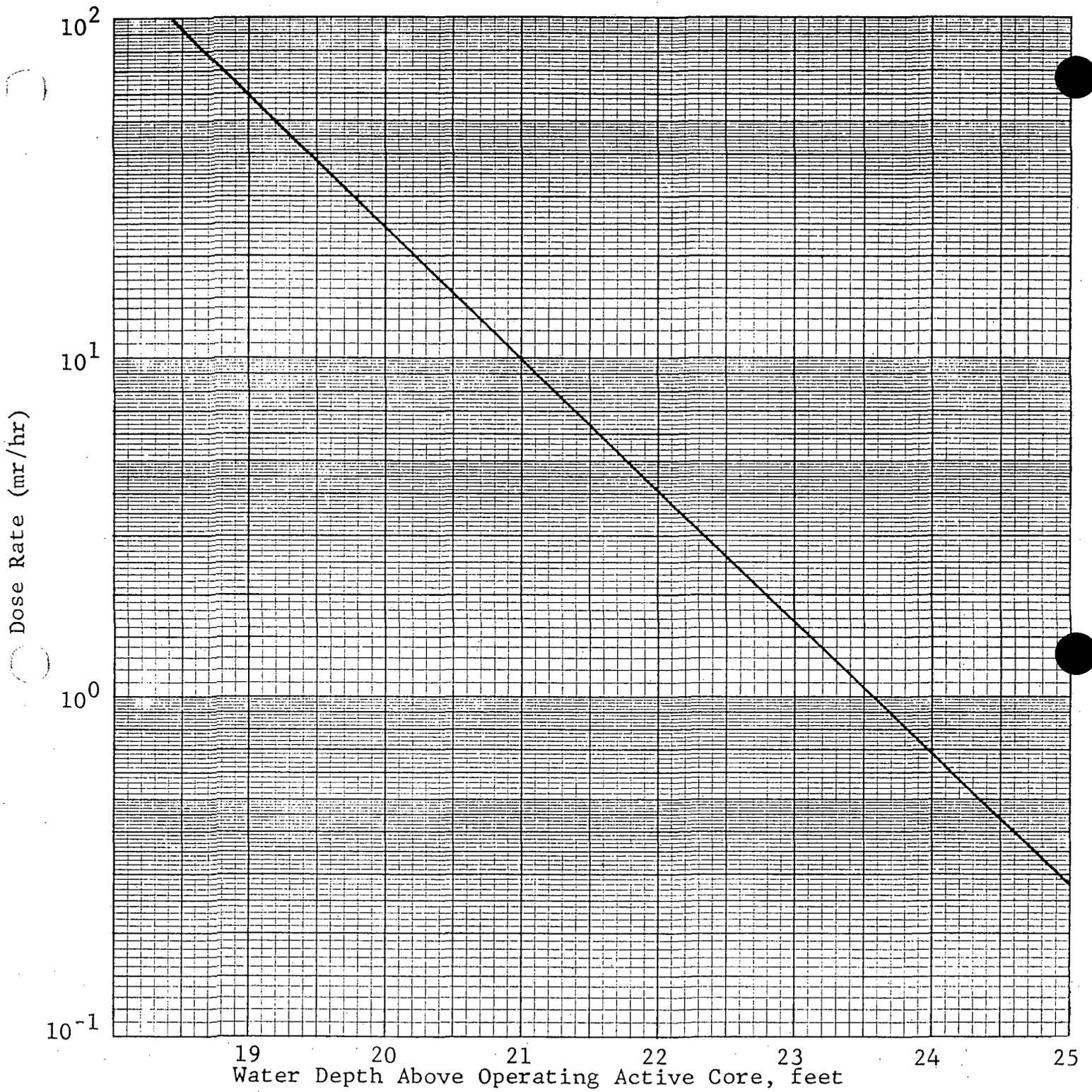
Figure 6.2 Direct Penetration Gamma Ray Dose Rates as a Function of Water Depth Above the Active Core Region (Reactor Power 10 MW)
