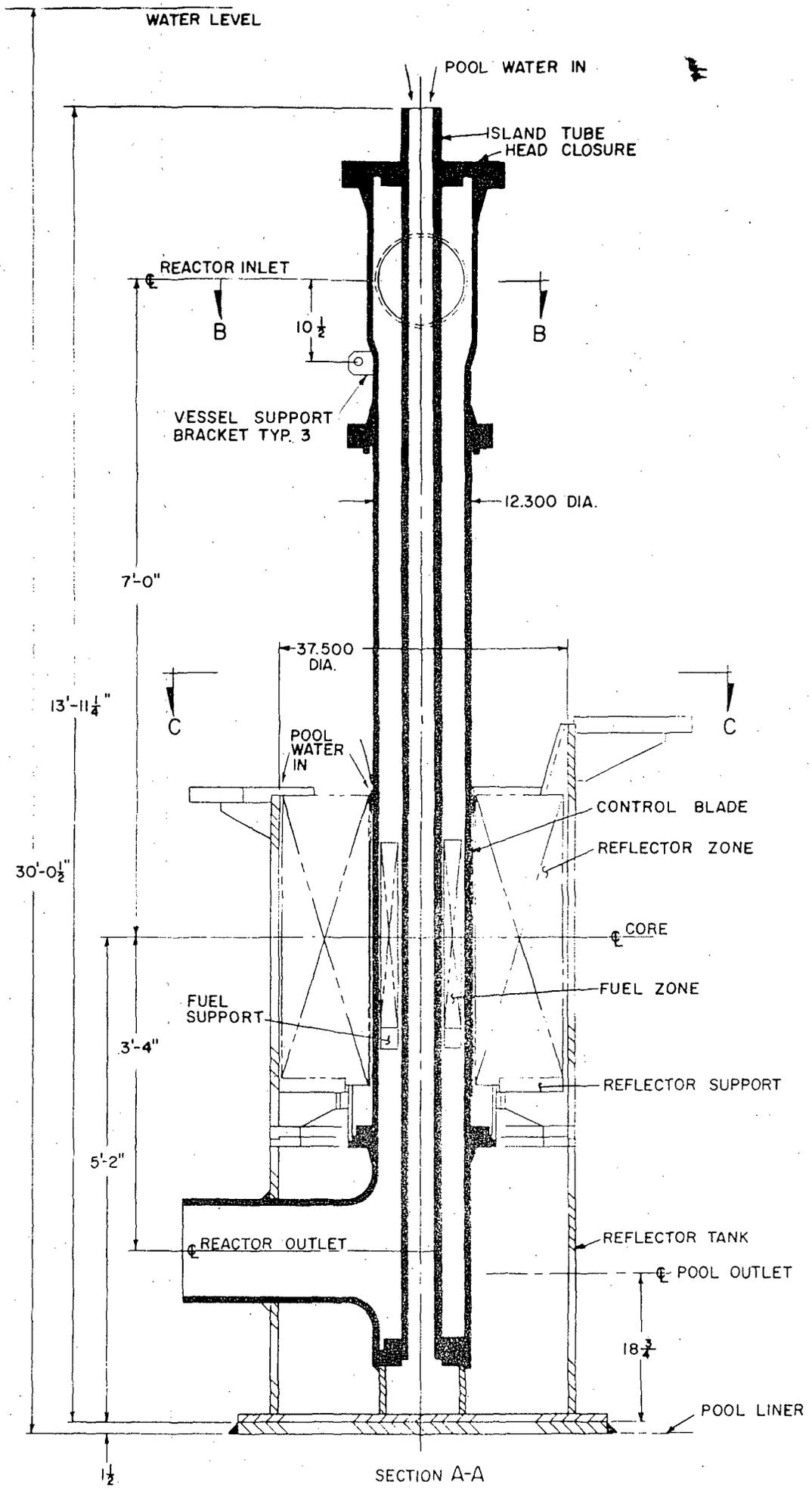
Figure 4.1 Reactor Assembly Section in Elevation View
