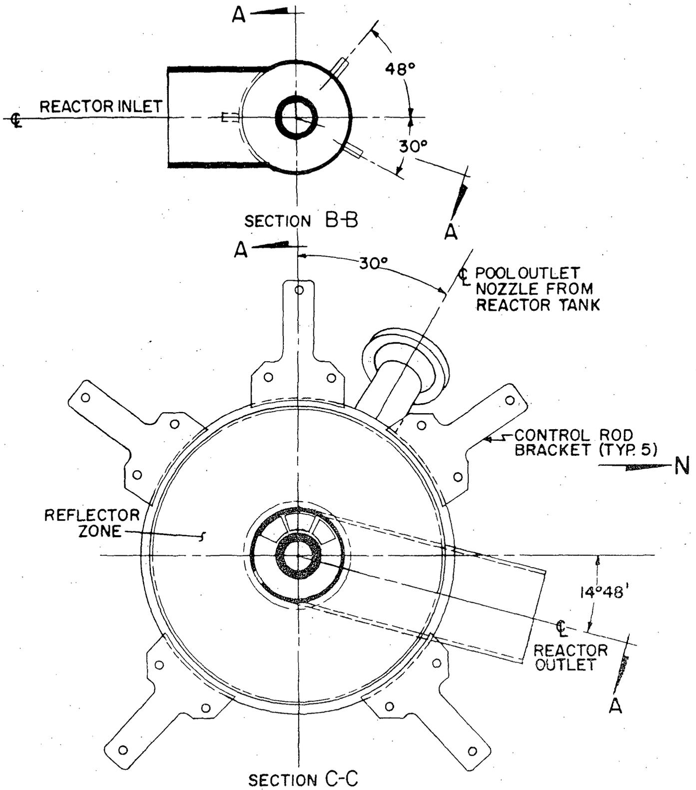
Figure 4.2 Reactor Assembly Sections in Plan View
