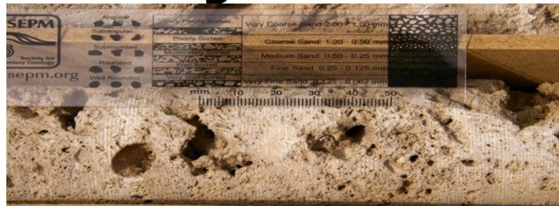
Small disconnected dissolution voids.
