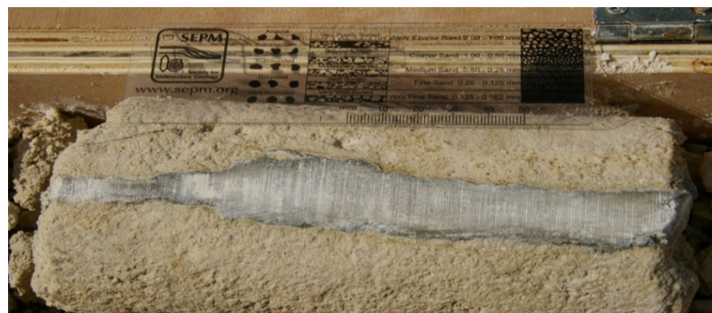
Grouted fracture sealed against fluid flow during grout testing.
