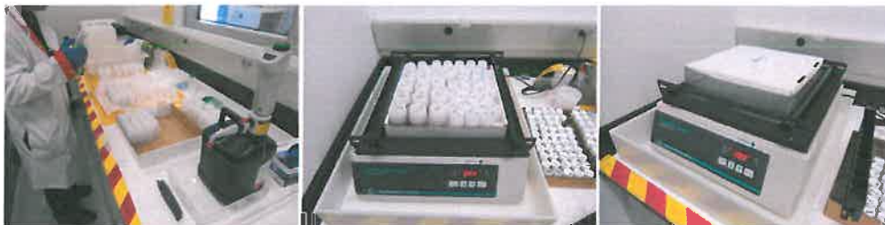
Figure 6 Placement of test samples in a container box and on the shaker table
