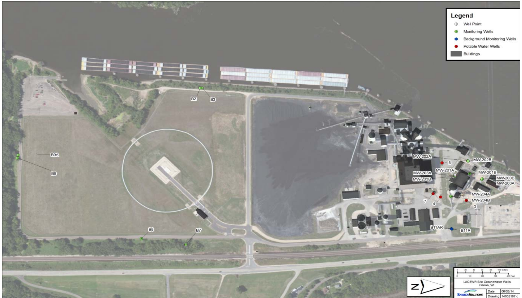
Figure 8-5 Groundwater Sampling Wells – LACBWR Site
