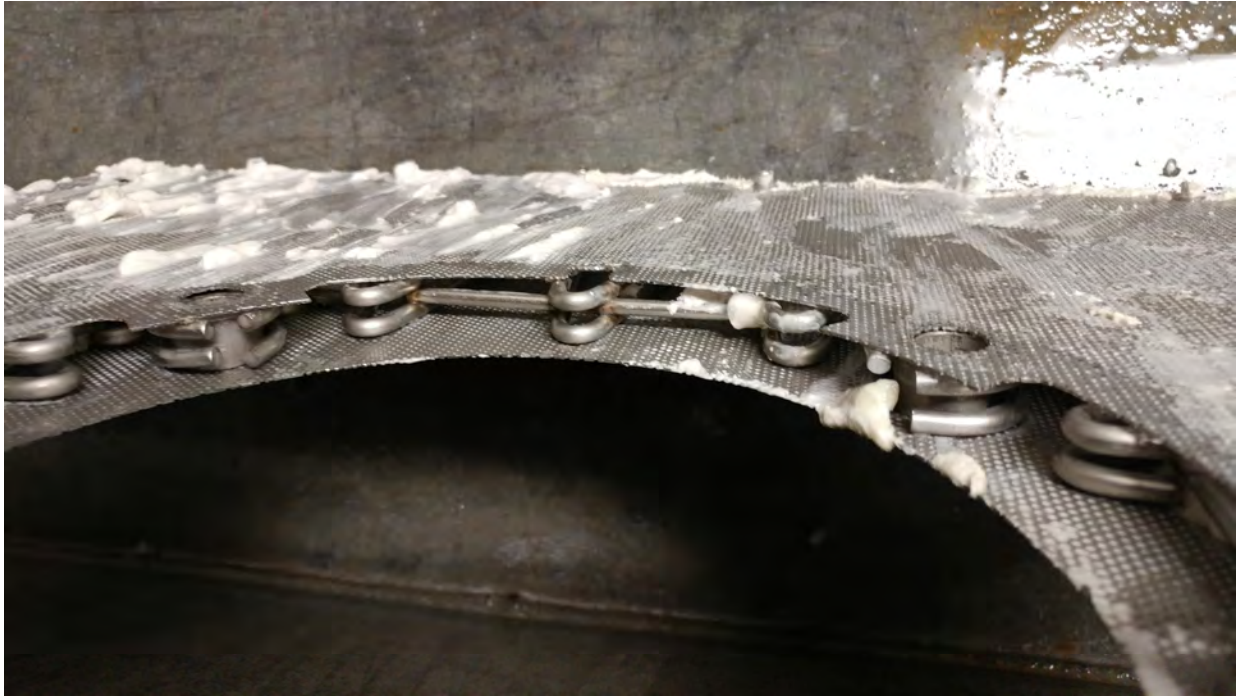
Photo 11 – Wire support structure for disks
