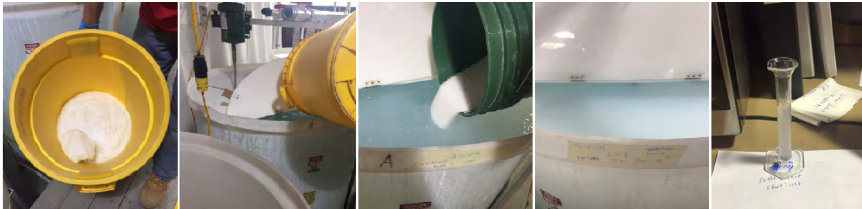
Photo 3 – Preparation of aluminum oxyhydroxide chemical precipitate debris
