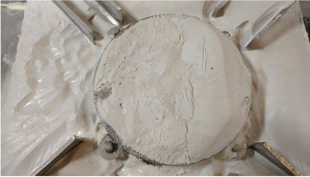
Photo 5 – Debris bed disturbed by gas release
