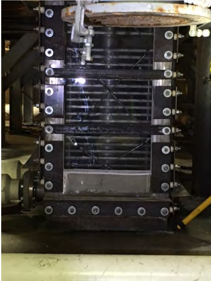
Photo 1 – Strainer in Test Tank
