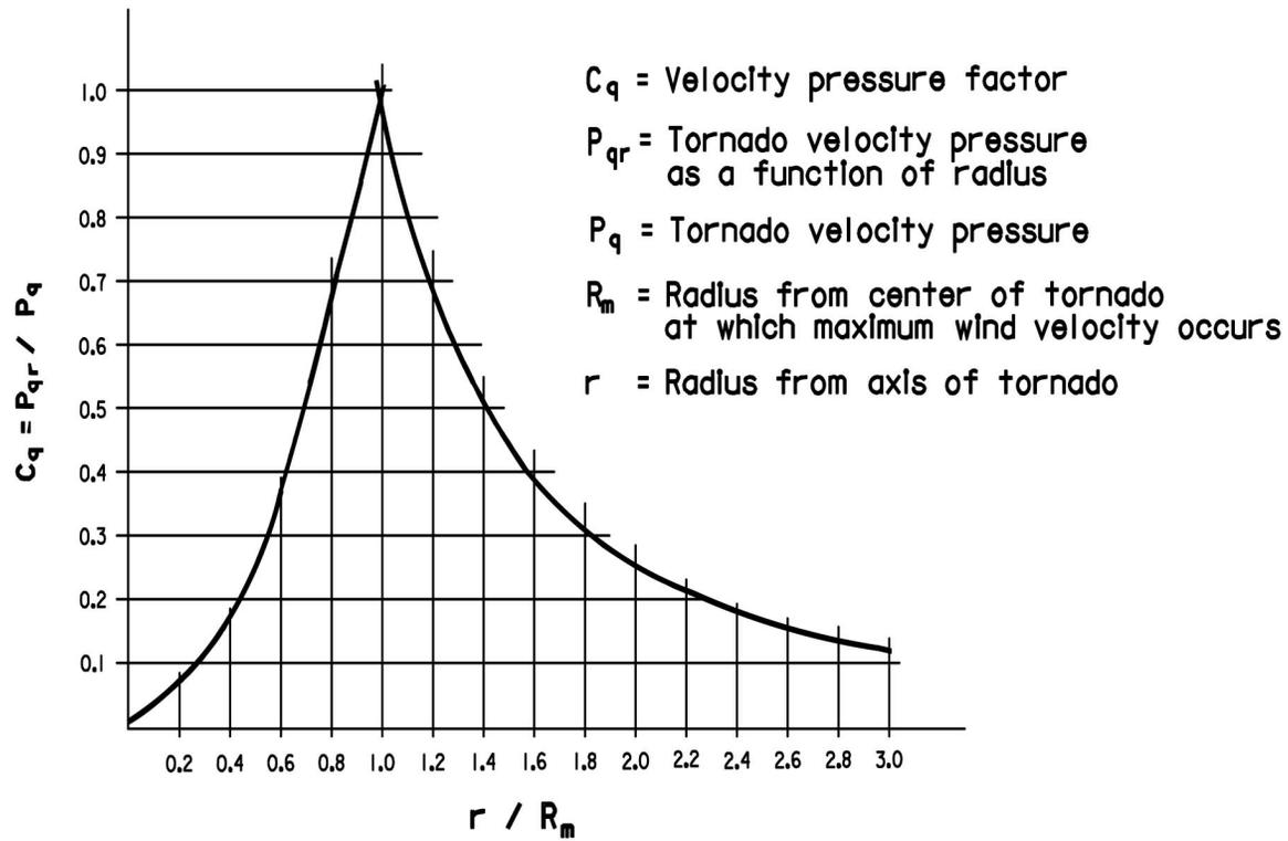
Figure 3.3-1 Velocity Pressure Variation with Radius from Center of Tornado
