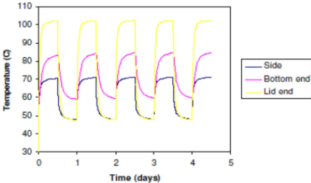
Figure 3-3 Predicted temperature on the Outside of the Keg During Normal Transport with Insulation
