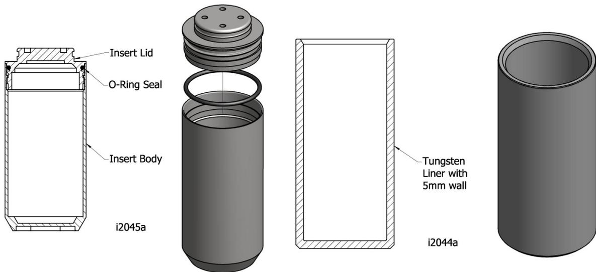
**Figure 1-5d Shielding insert HS-50x85-SS– Design # 4081 with Tungsten liner**
