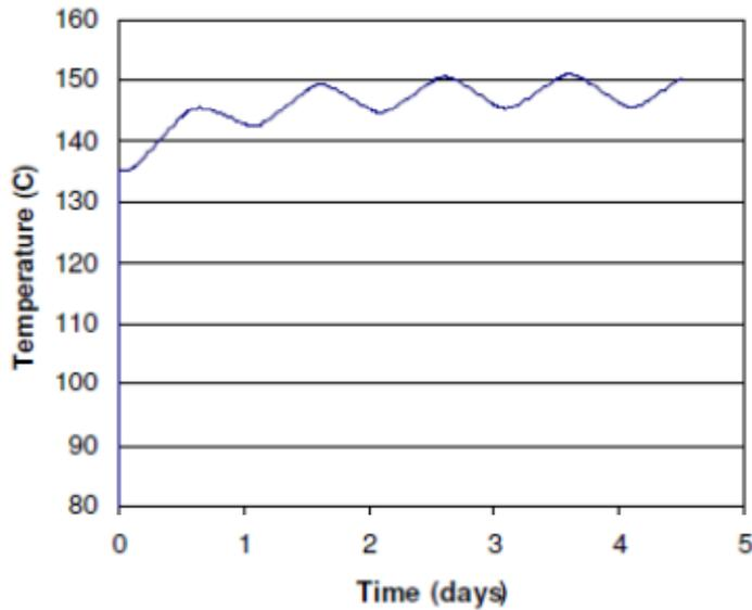
Figure 3-4 Predicted Temperature at the Containment vessel lid Seal During Normal Conditions of Transport with Insulation
