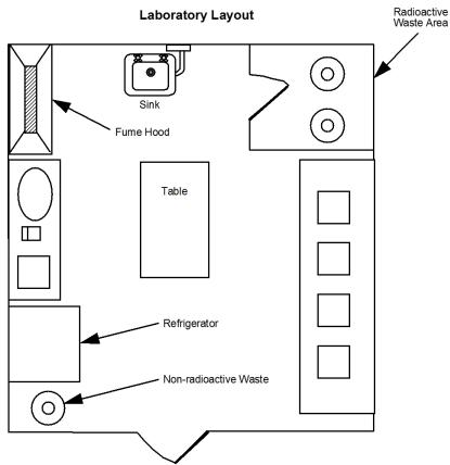
**Figure N–1. Laboratory Layout.** This is an example of a laboratory survey map.
