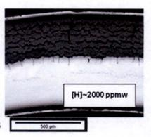
Comparison of uncoated and chromium coated Zircaloy-4 (Zy-4) samples after exposure to 1000 °C steam for 15000s by Cr-Coated Zy-4 metallographic cross-section and post-quench mechanical behavior.
