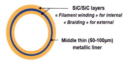
Candidate materials for liner selected on thermochemical and neutronic criteria : Ta, Nb (GFR)
