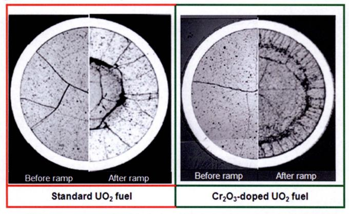
Post ramp ceramographs of Cr<sub>2</sub>O<sub>3</sub> doped UO<sub>2</sub> fuel and the reference UO<sub>2</sub> fuel
