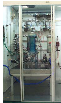
Lab Scale 2-inch CVD Coating (60 g charge)
