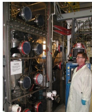
Industrial Scale 6-inch CVD Coating (2 kg charge)
