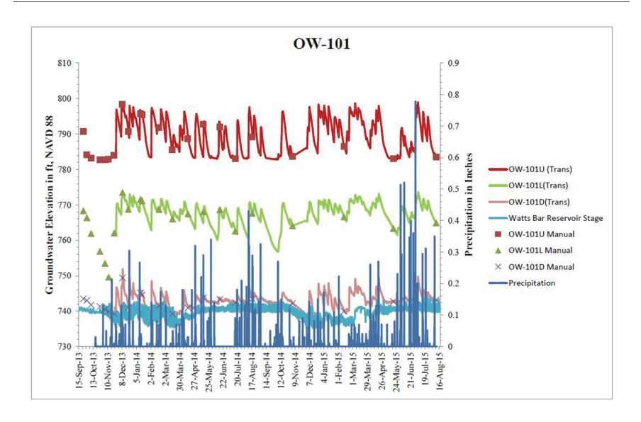
Figure 2.3.1-31. Hydrograph of OW-101 Well Cluster (Sheet 1 of 14)
