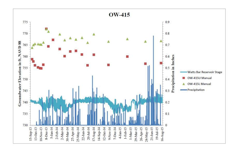
Figure 2.3.1-31. Hydrograph of OW-415 Well Cluster (Sheet 5 of 14)
