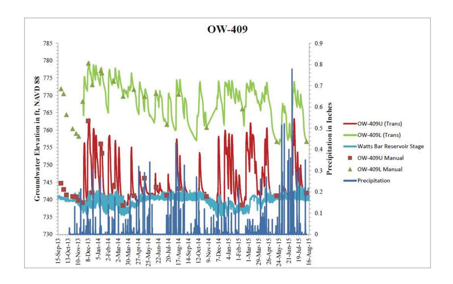
Figure 2.3.1-31. Hydrograph of OW-409 Well Cluster (Sheet 4 of 14)
