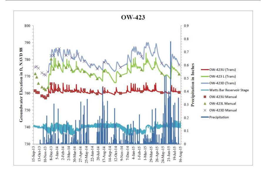
Figure 2.3.1-31. Hydrograph of OW-423 Well Cluster (Sheet 12 of 14)
