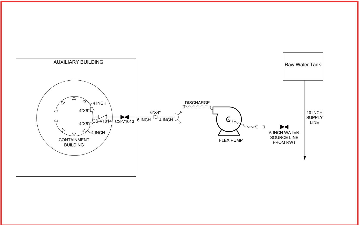
Figure 6-7 Flow Path for FLEX Connection to Deliver Water to Containment for ECSBS
