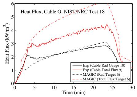
C.6.7 Surface Temperature and Surface Heat Flux
