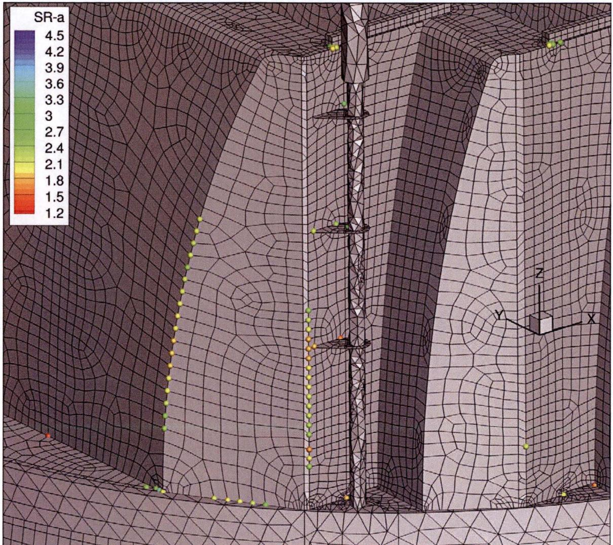
Figure 6d. Alternating stress ratios on welds [ [
