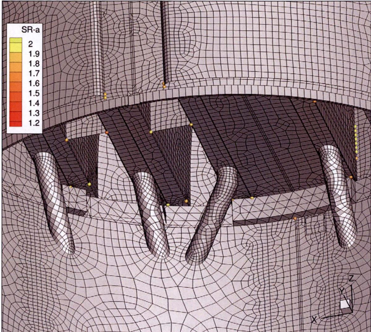
Figure 5e. Nodes on welds with alternating stress ratios below 2.1 on the NMP2 steam dryer [(<sup>3</sup>)]. Close-up view 5 of drain channel/skirt welds and various welds underneath dryer.
