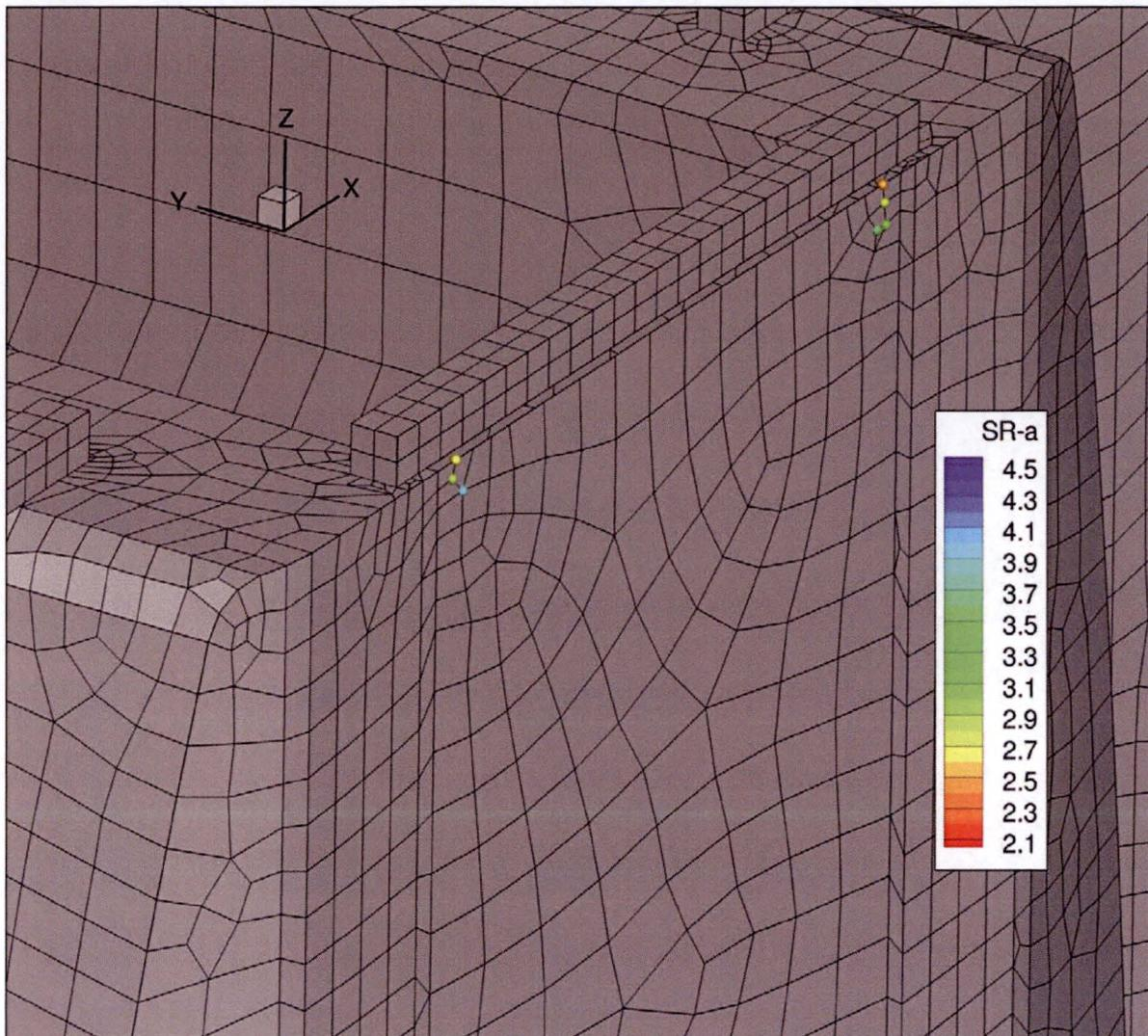
Figure 4d. Alternating stress ratios on non-weld locations [[
