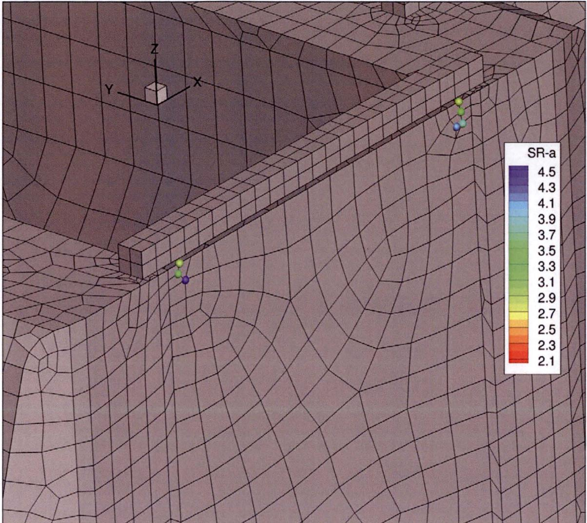
Figure 1d. Non-weld locations with alternating stress ratios below 4.5 on the NMP2 steam dryer [(3)]. Close-up view 4 of inner plate.
