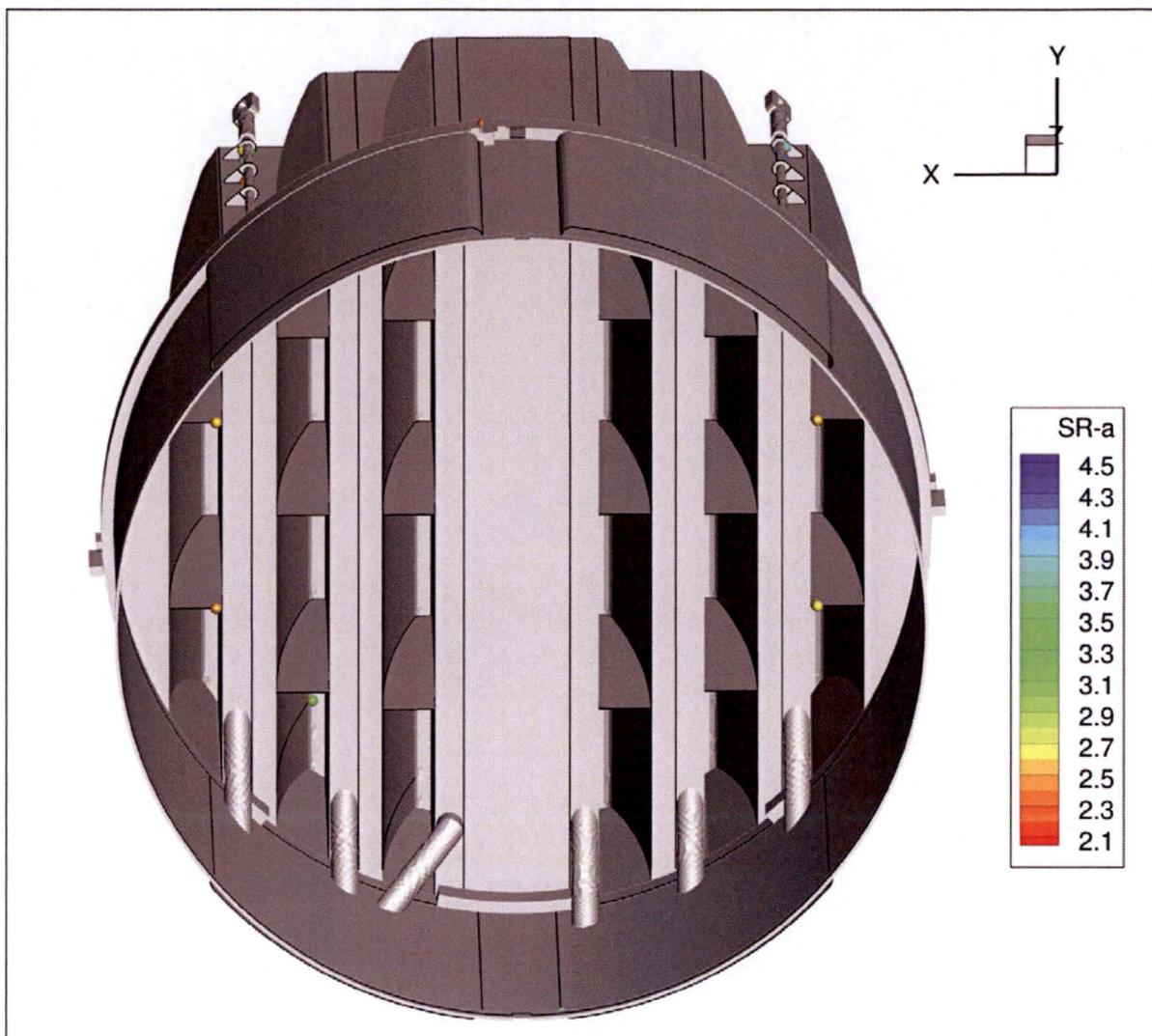
Figure 4b. Alternating stress ratios on non-weld locations [[
