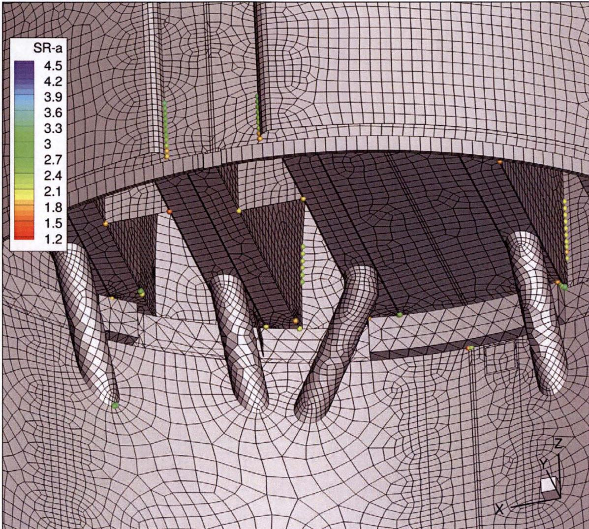
Figure 6e. Alternating stress ratios on welds [[
