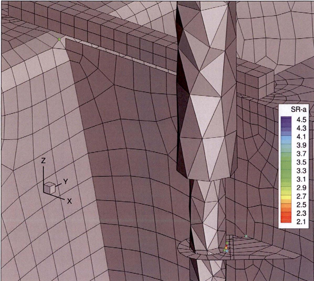
Figure 4c. Alternating stress ratios on non-weld locations [[
