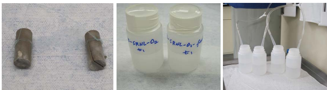
Figure 4.1. The Cast Stone Monoliths Without and With Fracture (left), Leaching Vessels of 125 mL Poly Bottles (middle), and Preparation of O 2 -Saturated Leaching Solution by Pure O 2 (g) Bubbling Used for the EPA 1315 Method Leach Test (right)
