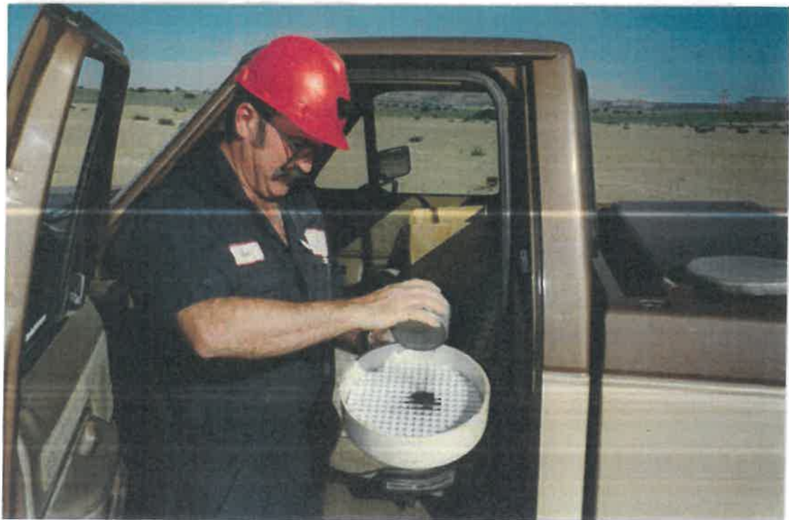
Photograph 4 - Environmental technician pouring charcoal into LAACC.
