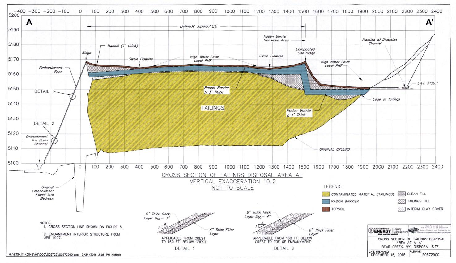
Figure 7. Tailings Embankment and Impoundment Cross Section
