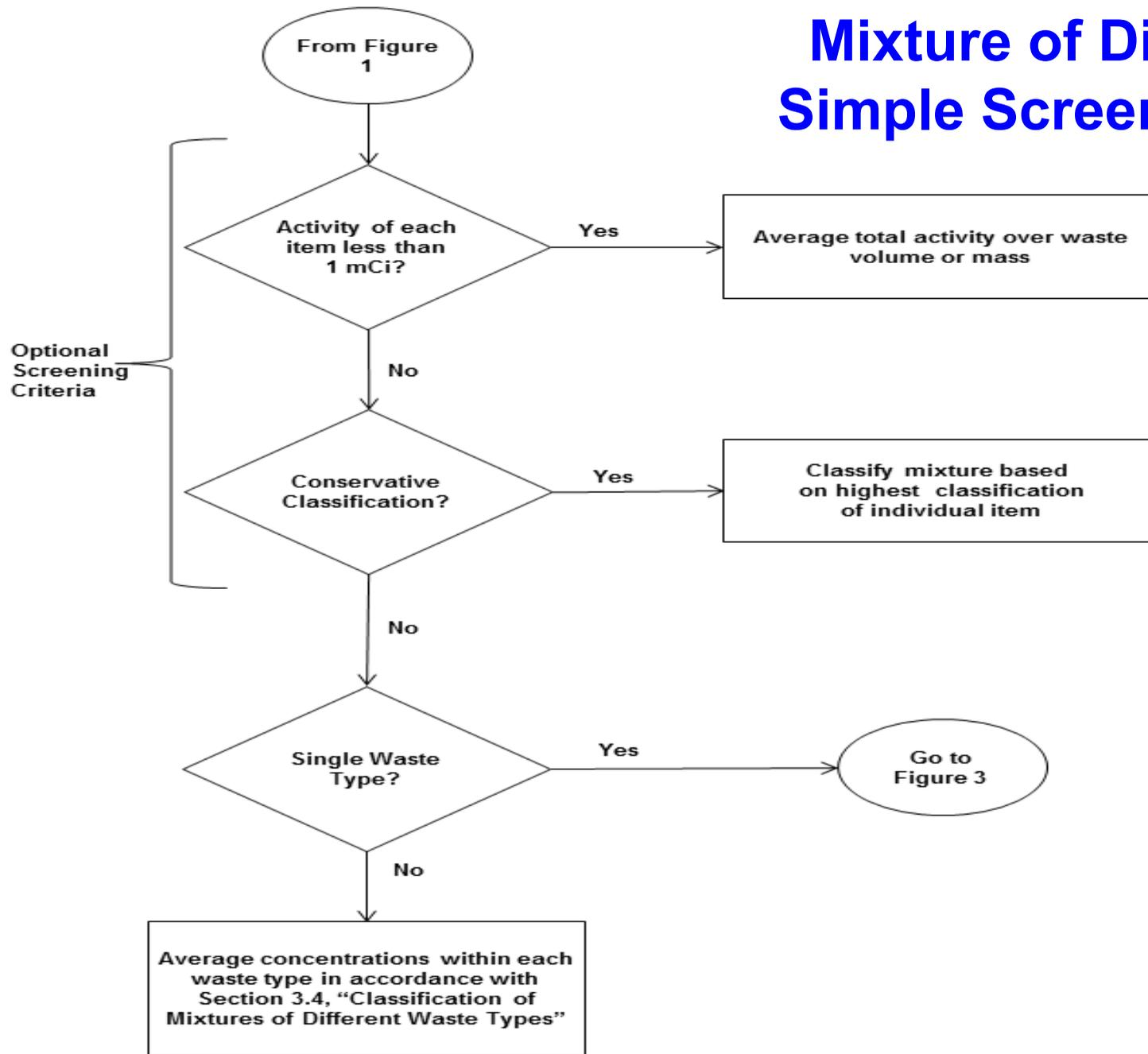
Figure 2. Overview of Classification of Mixtures of Discrete Items (Sections 3.3.2.1 and 3.3.2.2)
