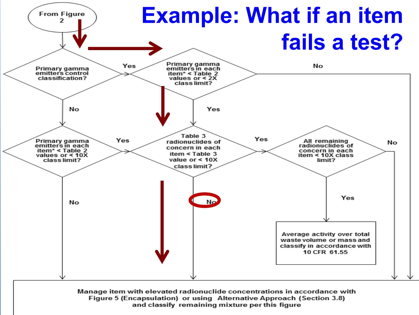
\* For comparison to Table 2 values, items larger than 280 cc (0.01 ft<sup>3</sup>) may be treated individually. Items smaller than 280 cc (0.01 ft<sup>3</sup>) should be grouped together (see Section 3.3.2.2).
