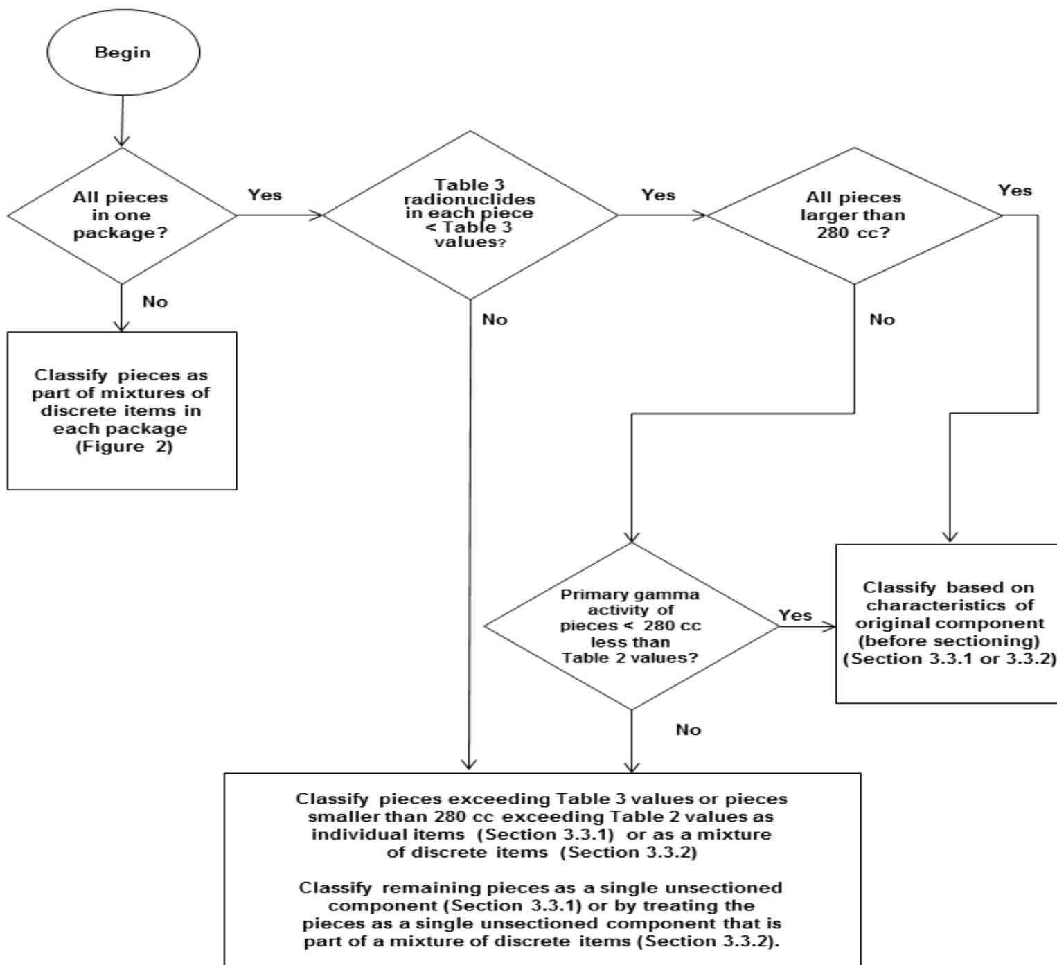
**Figure 4. Classification of Sectioned Components (from Section 3.3.2.3)**
