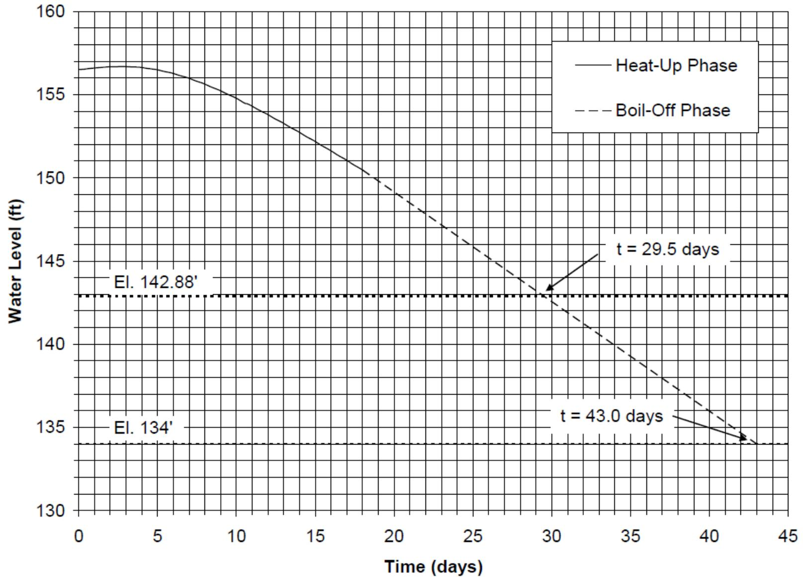
Figure 3.7-2: Extended SFP Water Level for Scenario inop-5y
