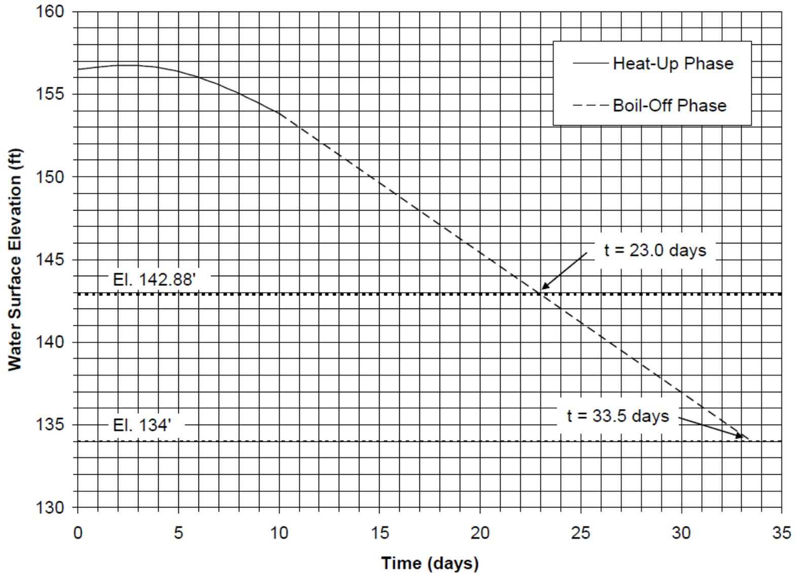
Figure 3.5-2: Extended SFP Water Level for Scenario inop-0y
