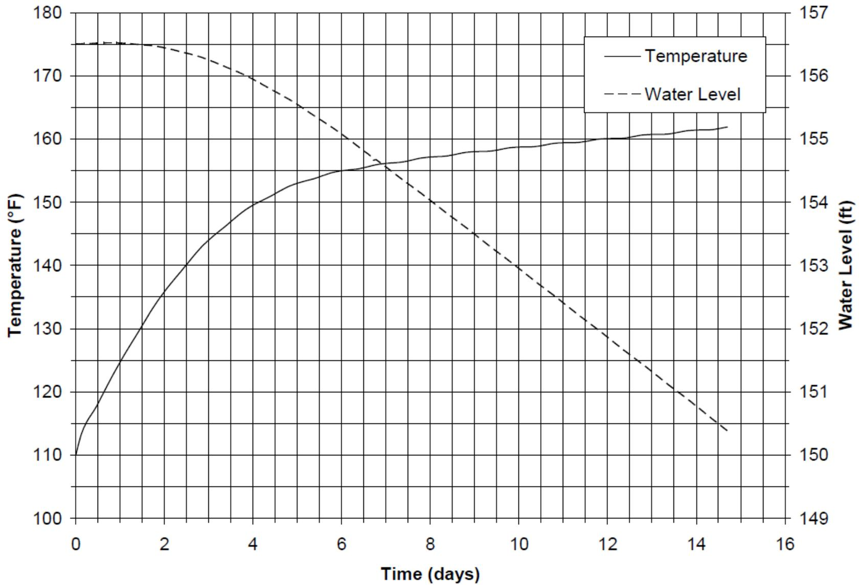
Figure 3.8-1: SFP Temperature and Level for Scenario op-5y
