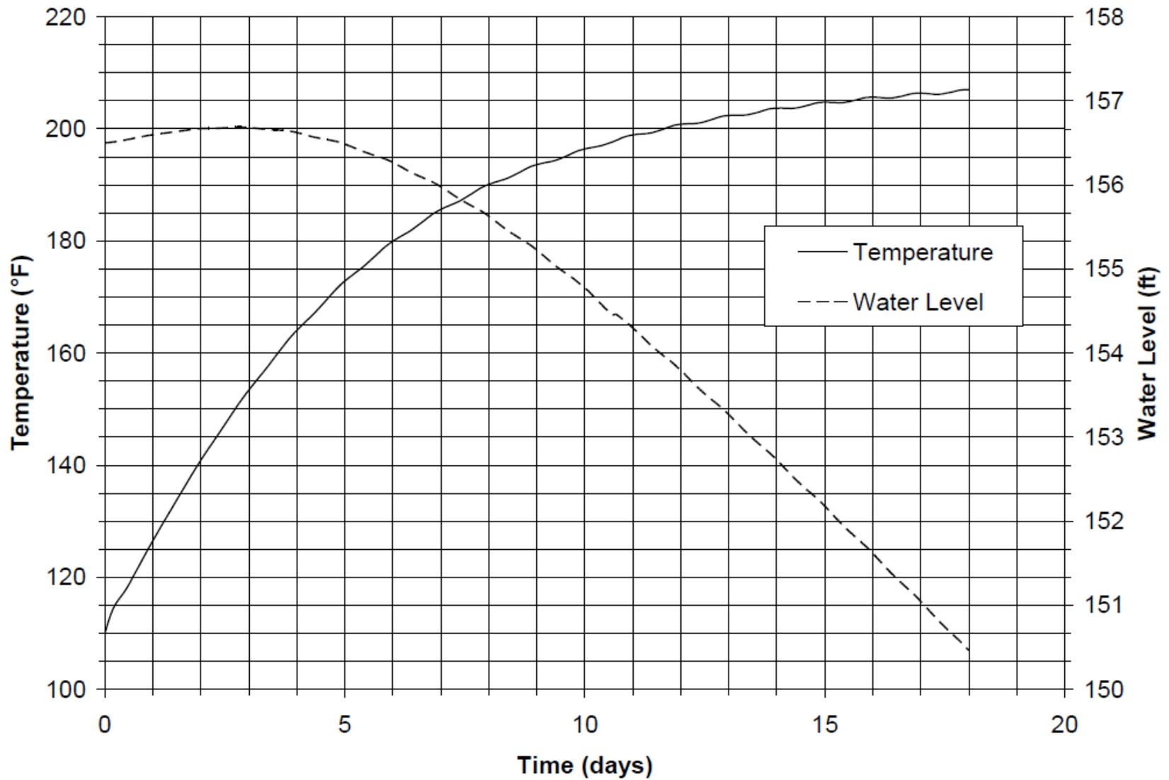
Figure 3.7-1: SFP Temperature and Level for Scenario inop-5y
