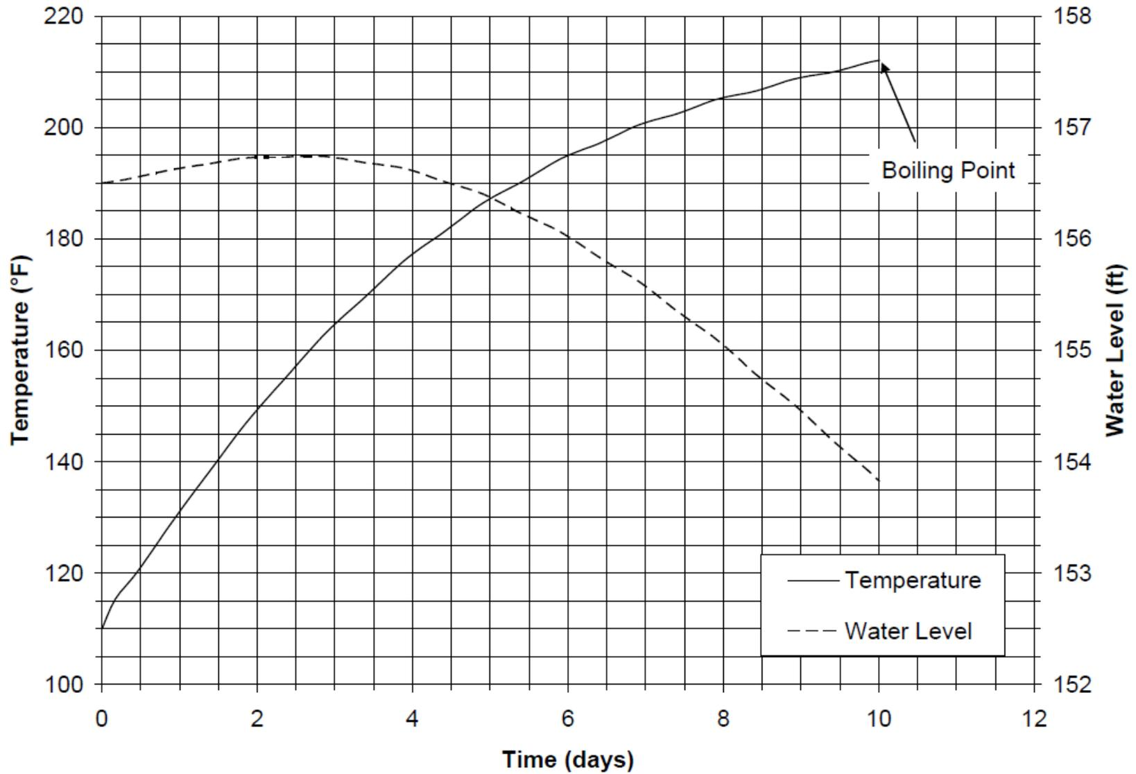
Figure 3.5-1: SFP Temperature and Level for Scenario inop-0y
