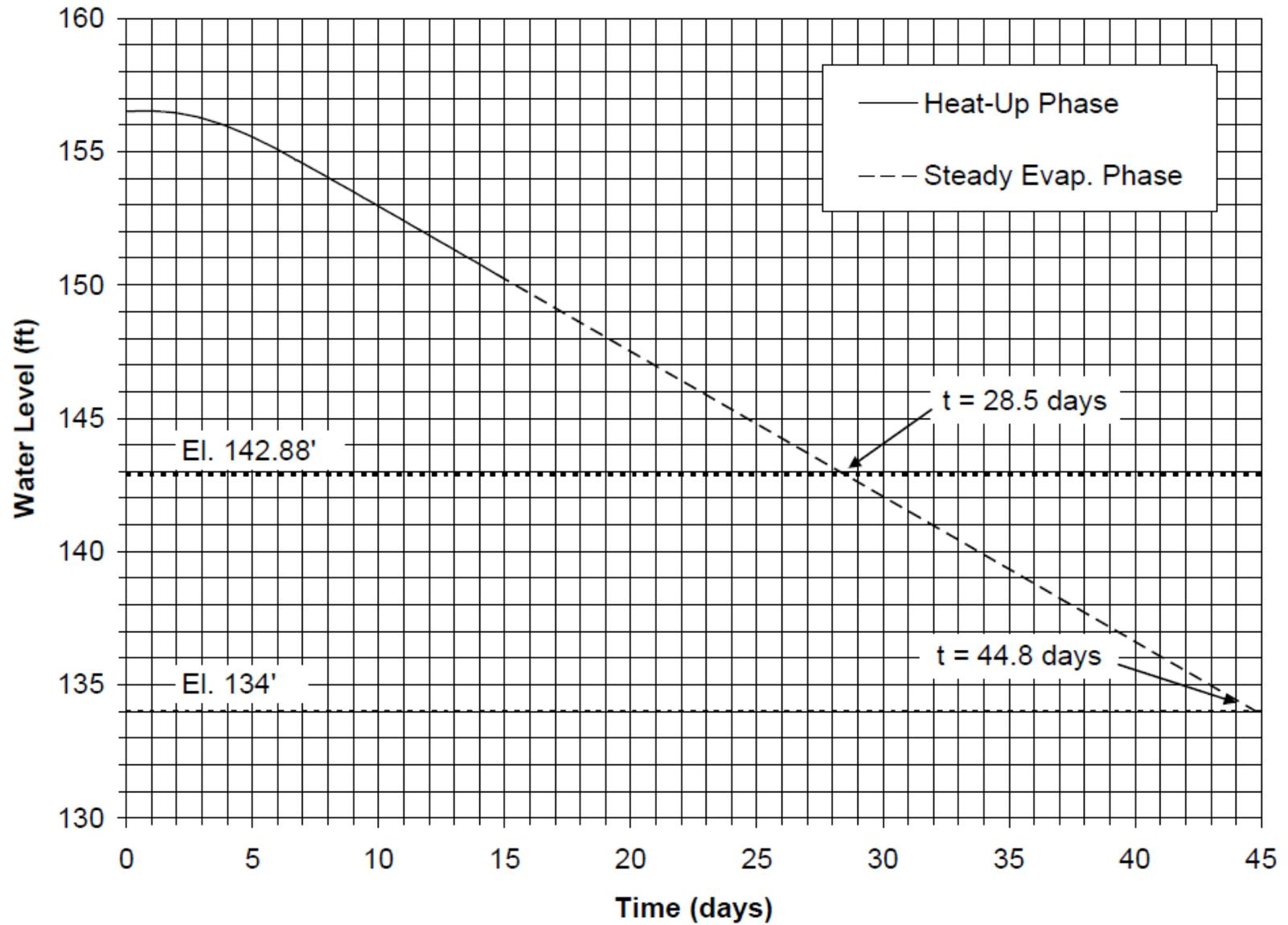
Figure 3.8-3: Extended SFP Water Level for Scenario op-5y
