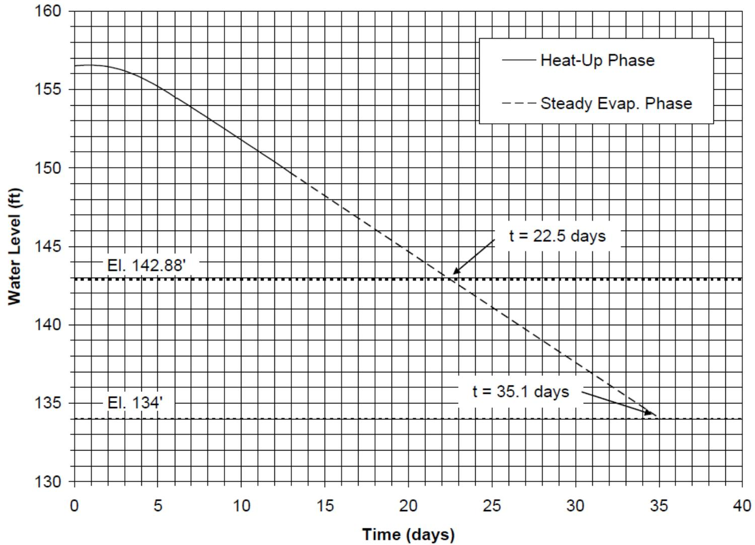
Figure 3.6-3: Extended SFP Water Level for Scenario op-0y
