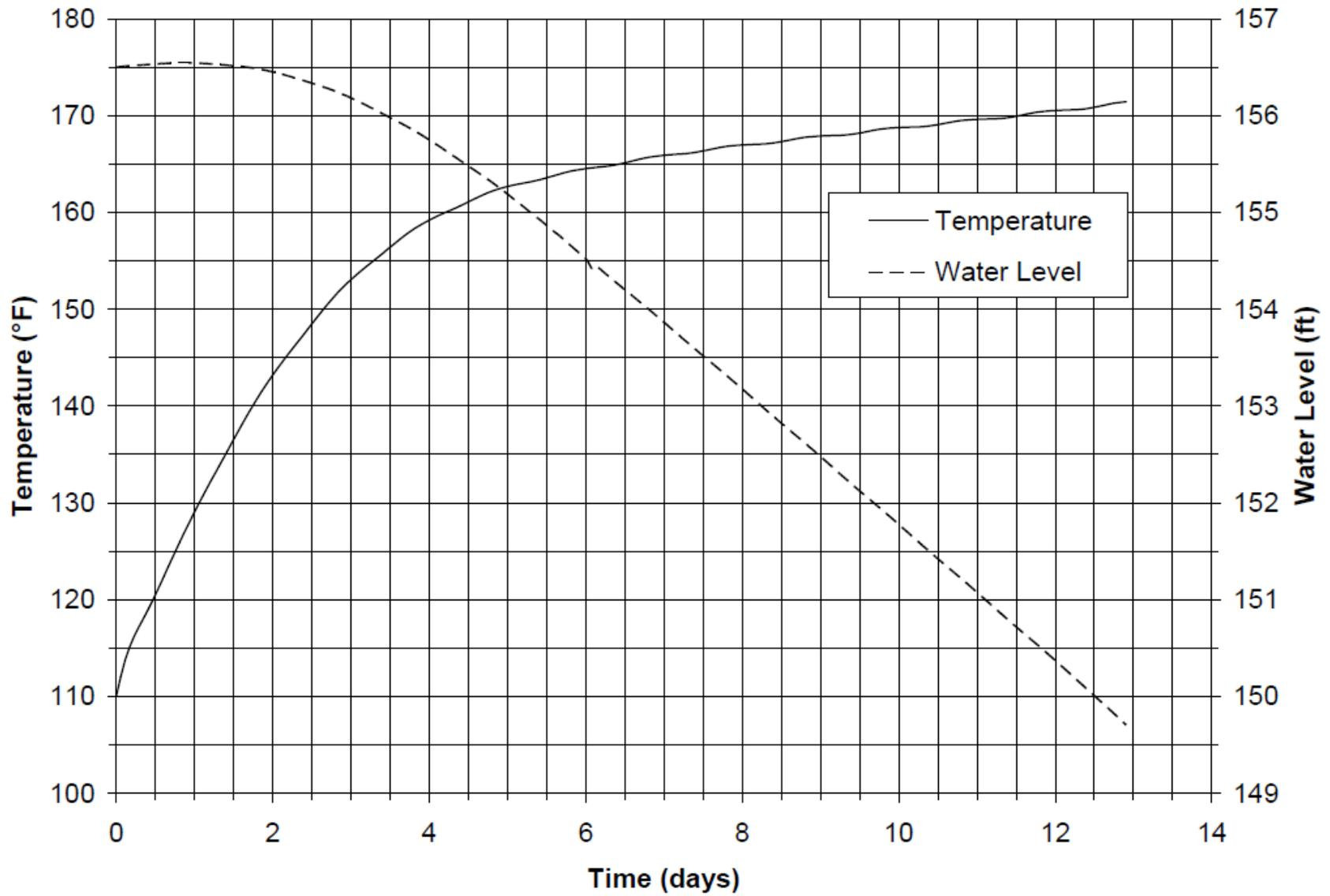
Figure 3.6-1: Extended SFP Water Level for Scenario op-0y
