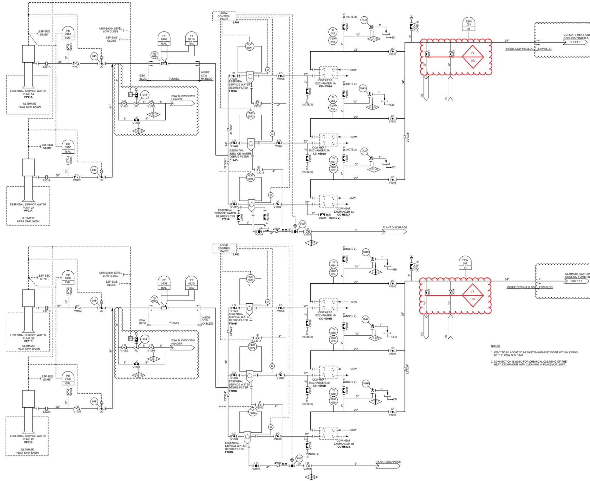
Figure 9.2.1-1 Essential Service Water System Flow Diagram
