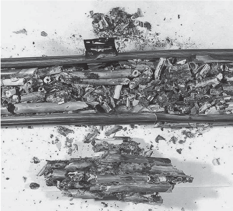
Figure 2. Section of the FLECHT Run 9573 Test Bundle that Incurred Runaway Oxidation
