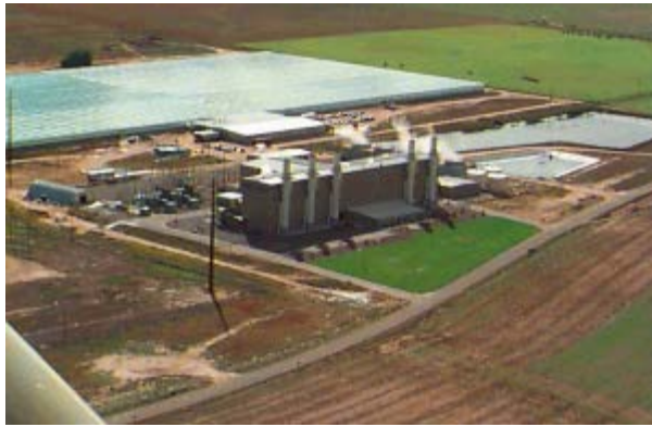
Combined-Cycle Power Plant and Steam-Host, 272 MW
