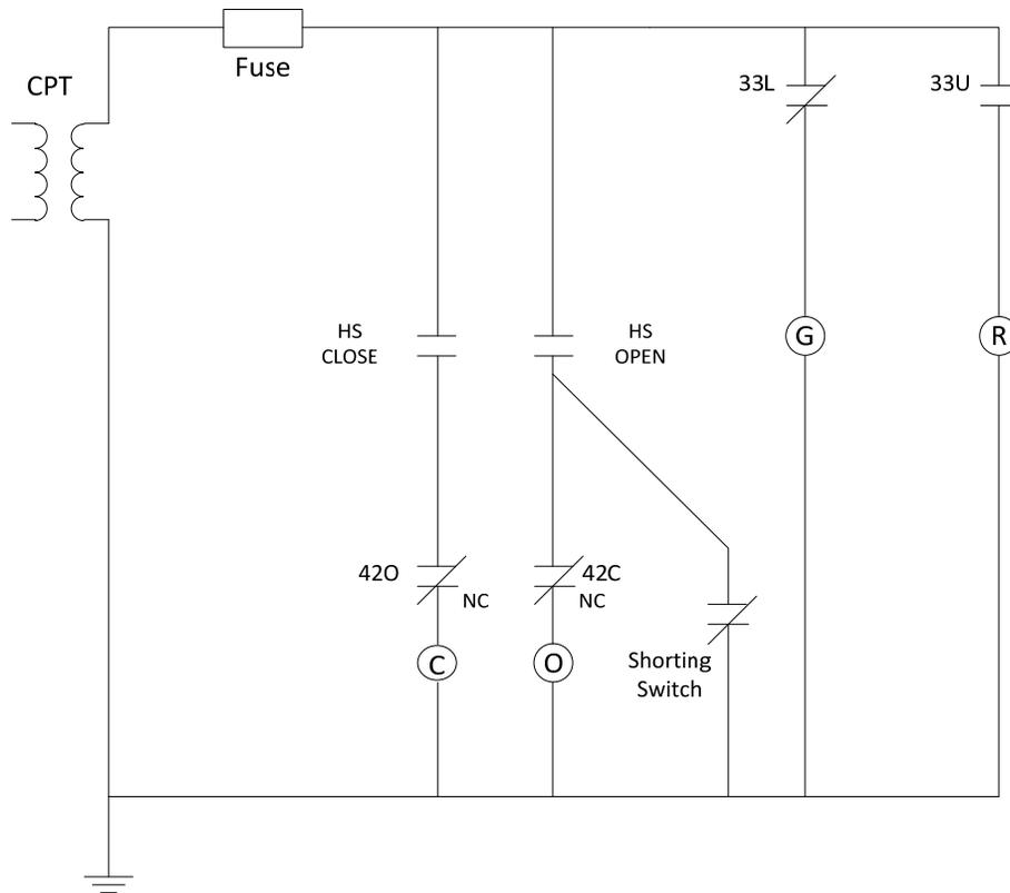
**Figure I.2.0 – Simplified MOV Circuit with Shorting Switch**
