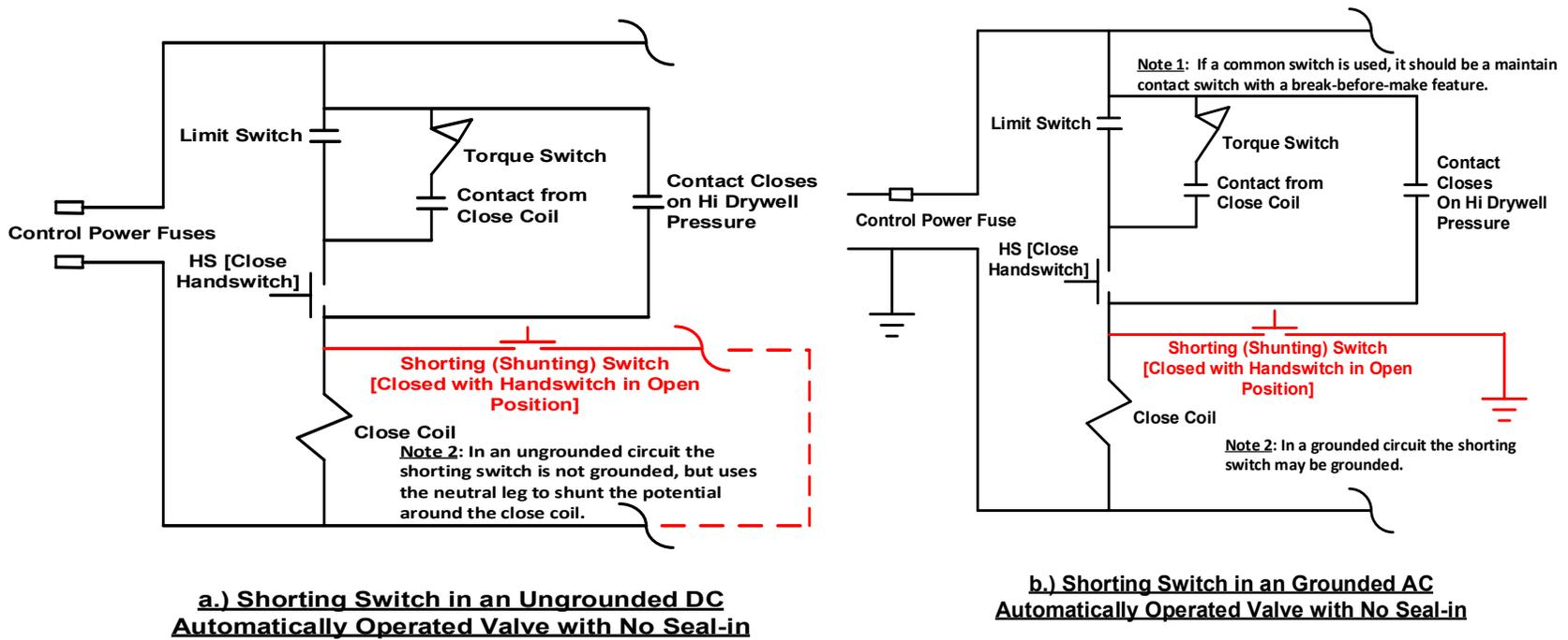
**Figure I.6.0– Simplified Illustration of Shorting Switch in Control Circuits With Automatic Control and Without Seal-In Features**
