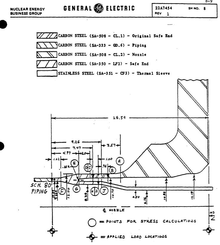
FIGURE 3.1 NOZZLE, SAFE END, AND THERMAL SLEEVE GEOMETRY
