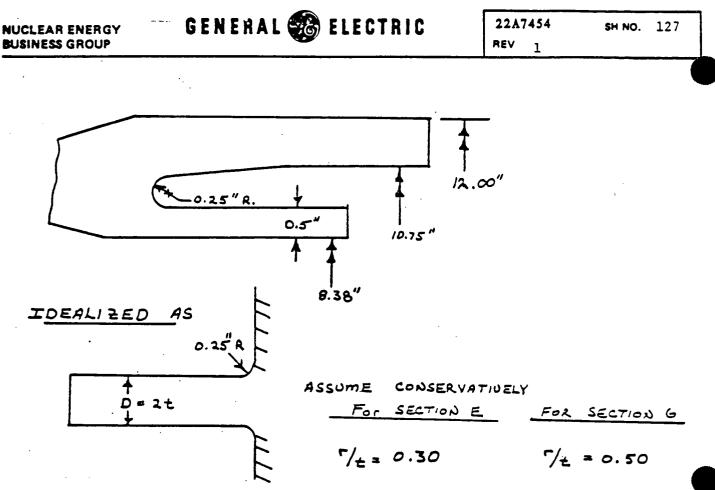
FIGURE 4.3-3 SECTION E AND G GEOMETRY
