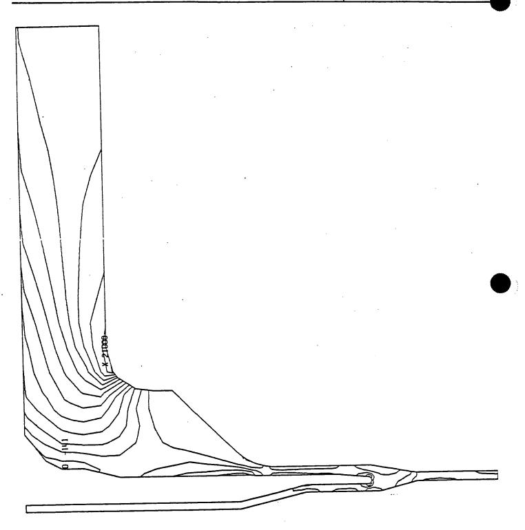
FIGURE 4.2.4-2 MONTICELLO FEEDWATER NOZZLE STRESS ANALYSIS - STRESS PLOT (PRESSURE RUN)
