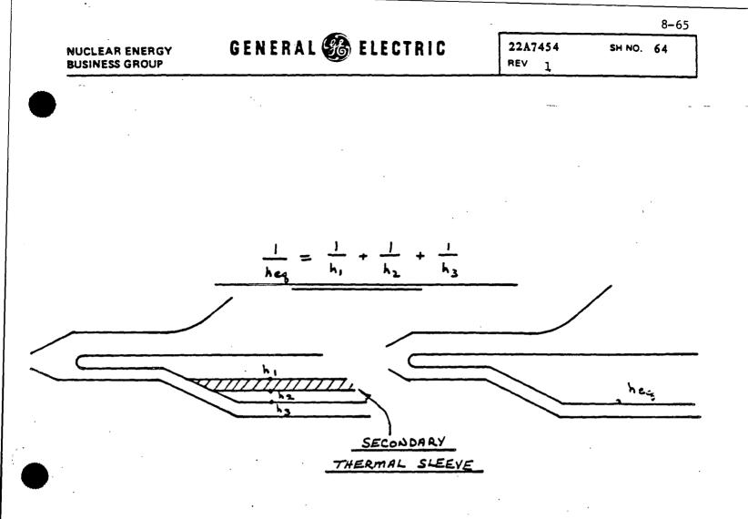
FIGURE 4.1.2-2 EQUIVALENT HEAT TRANSFER COEFFICIENT
