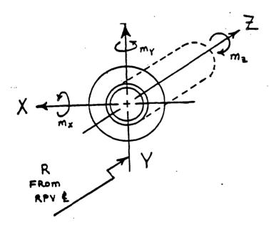
Sign Convention applies to both safe end and thermal sleeve loadings.
