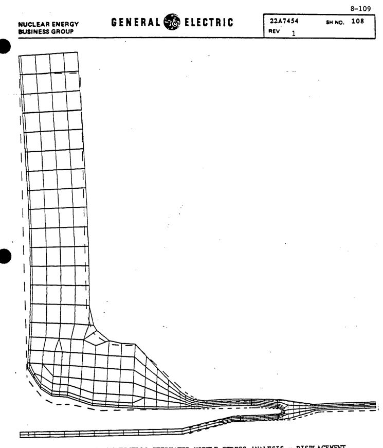
FIGURE 4.2.4-1 MONTICELLO FEEDWATER NOZZLE STRESS ANALYSIS - DISPLACEMENT PLOT (PRESSURE RUN)
