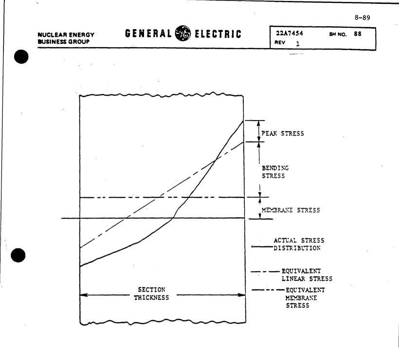
LINEARIZATION OF STRESS DISTRIBUTION ACROSS A SECTION THICKNESS
