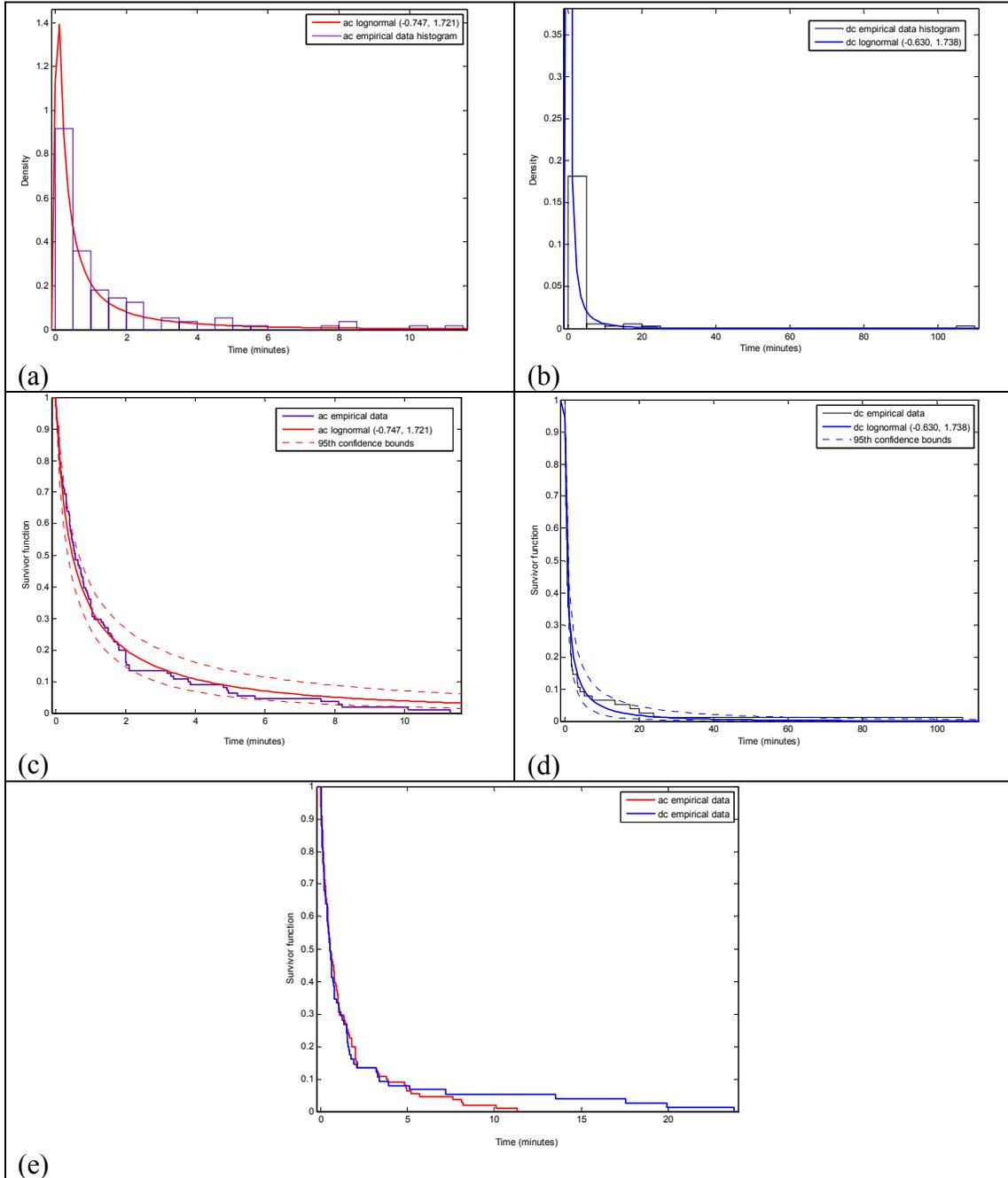
**Figure 1. Empirical data and parametric distributions for AC and DC spurious operation duration. Histogram and probability density function (a, b), empirical and distribution survivor function (c,d), empirical data survivor function (e).**
