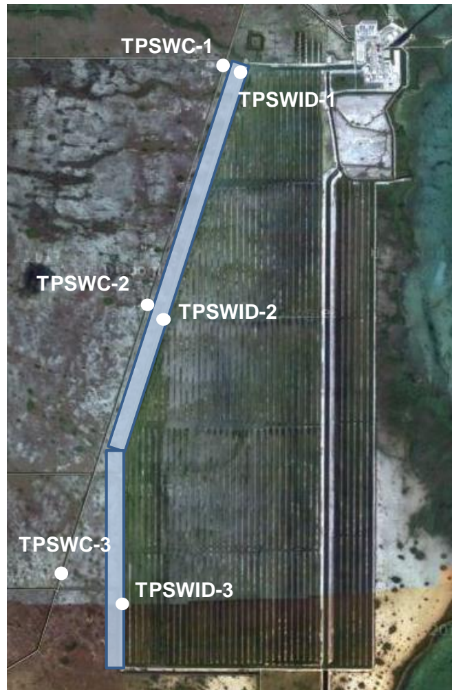
Figure 5.4-3. Locations of L-31E and ID Monitoring Stations; Conceptualized Seepage from L-31E into the ID is Shown.
