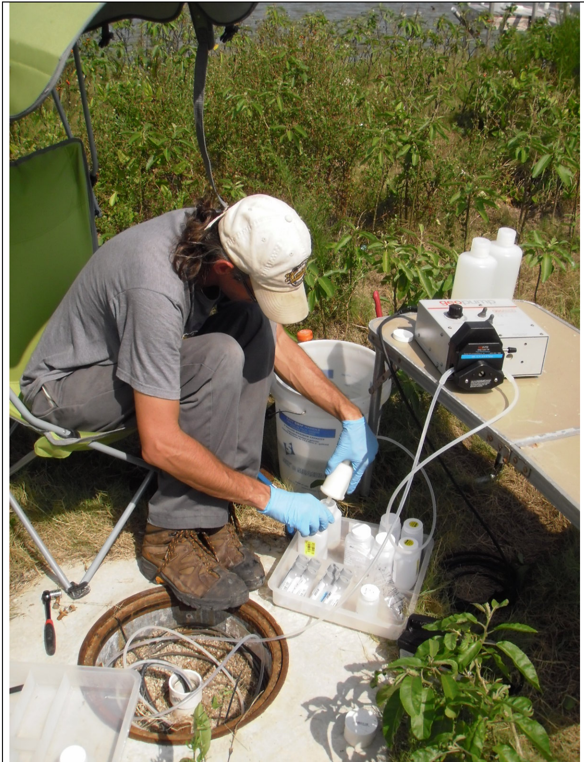
Figure 3.1-1. Typical Groundwater Field Sampling Setup.
